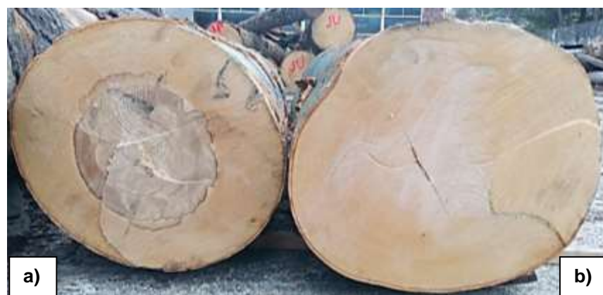
Fig. 1. a) Log with healthy red false heartwood and b) log without any type of red false heartwood
