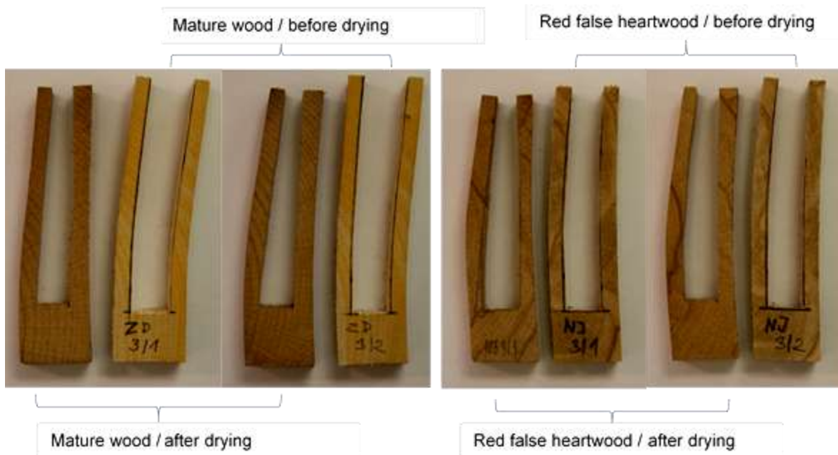
Fig. 7. Prong samples before and after drying
