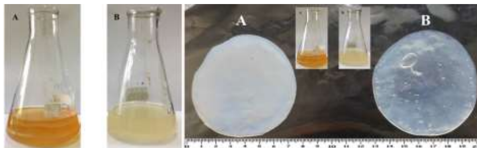
Fig. 3. Culture medium of yeast extract (A), and rice bran (B), and the respective harvested cellulose
