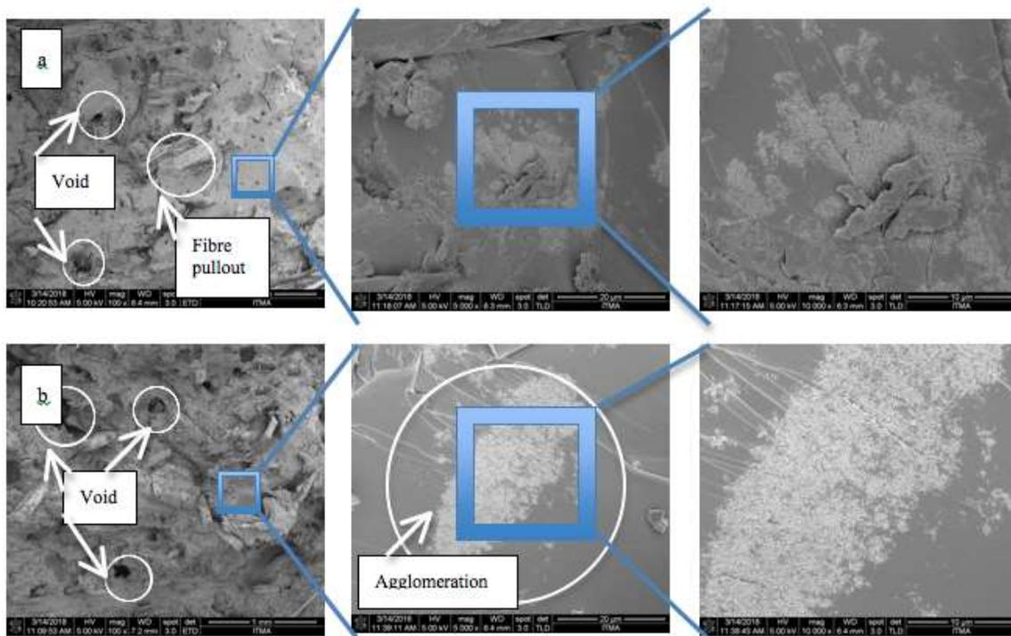
**Fig. 4.** FE-SEM image of fracture surface of (a) 0.5 wt.% CNTs, and (b) 1.0 wt.% CNTs
