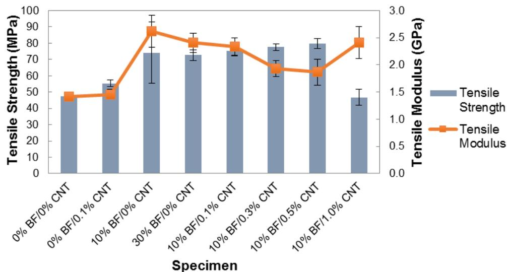
**Fig. 3.** Tensile modulus and tensile strength of bamboo/glass fibre hybrid composites enhanced with CNTs
