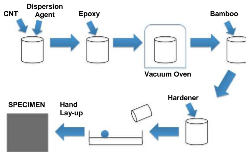
Fig. 1. Schematic of composite fabrication
