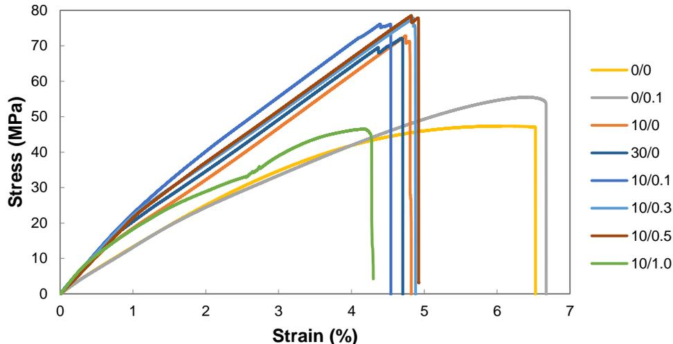
**Fig. 2.** Tensile stress-strain curves of bamboo/glass fibre hybrid composites enhanced with CNTs
