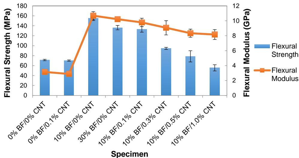
**Fig. 5.** Flexural modulus and flexural strength of bamboo/glass fibre hybrid composites enhanced with CNTs
