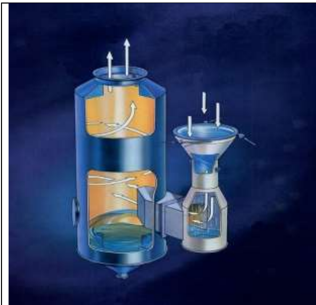
Fig. 19. Venturi Scrubber (Source: AirPol, Inc.); figure used with permission of the copyright holder.
