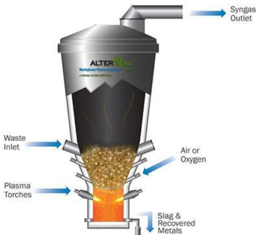
Fig. 16. Plasma Gasifier (Source: Alter NRG Corp.); figure used with permission of the copyright holder.
