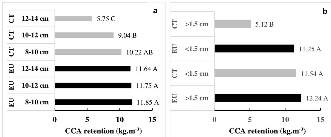
**Fig. 2.** CCA retention according to (a) diameter and (b) radial position. Similar capital letters on the same chart mean no statistical difference among the treatments by LSD test; p > 0.005.
