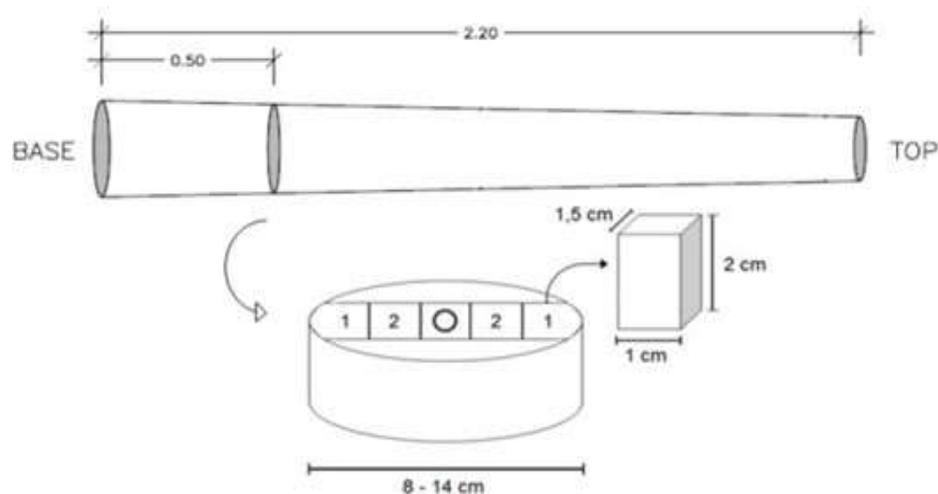
Fig. 1. Region of the fence post where the disk was taken and sample dimensions
