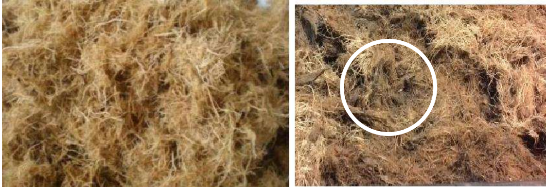
Fig. 2. OPEFB before (left) and OPEFB after the steam pretreatment (right)
