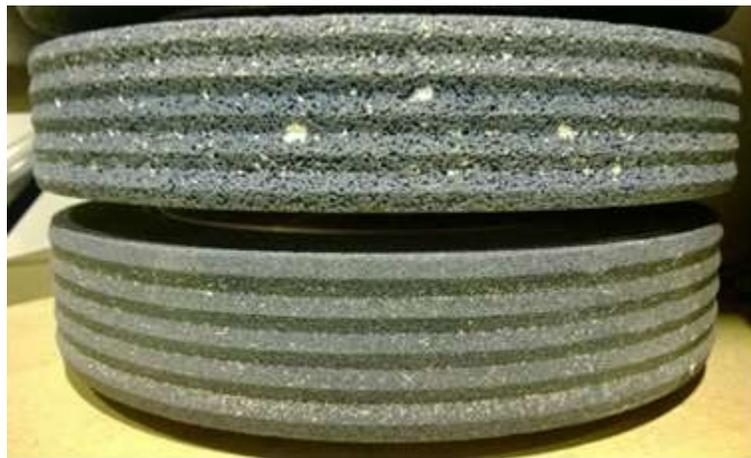
**Fig. 3.** The modified grinding stone surfaces applied in the experiments. The upper stone has a more porous structure than the lower one. The width of the stone is 50 mm and the diameter is 300 mm. The distance of the serrated pattern tops is 10 mm and the serrated angle is 15 degrees (see Fig. 1). The depth of the serrated valley is 1.4 mm.
