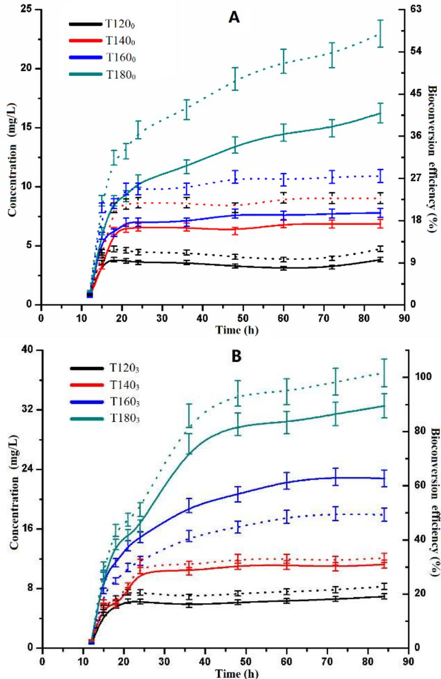
**Fig. 2.** Variation of glucose concentration (solid lines, left axis) and bioconversion efficiency (dotted lines, right axes) during 72 h enzyme hydrolysis for different pretreatment temperatures and incubation periods (A: incubation time = 0 h; B: incubation time = 3 h)
