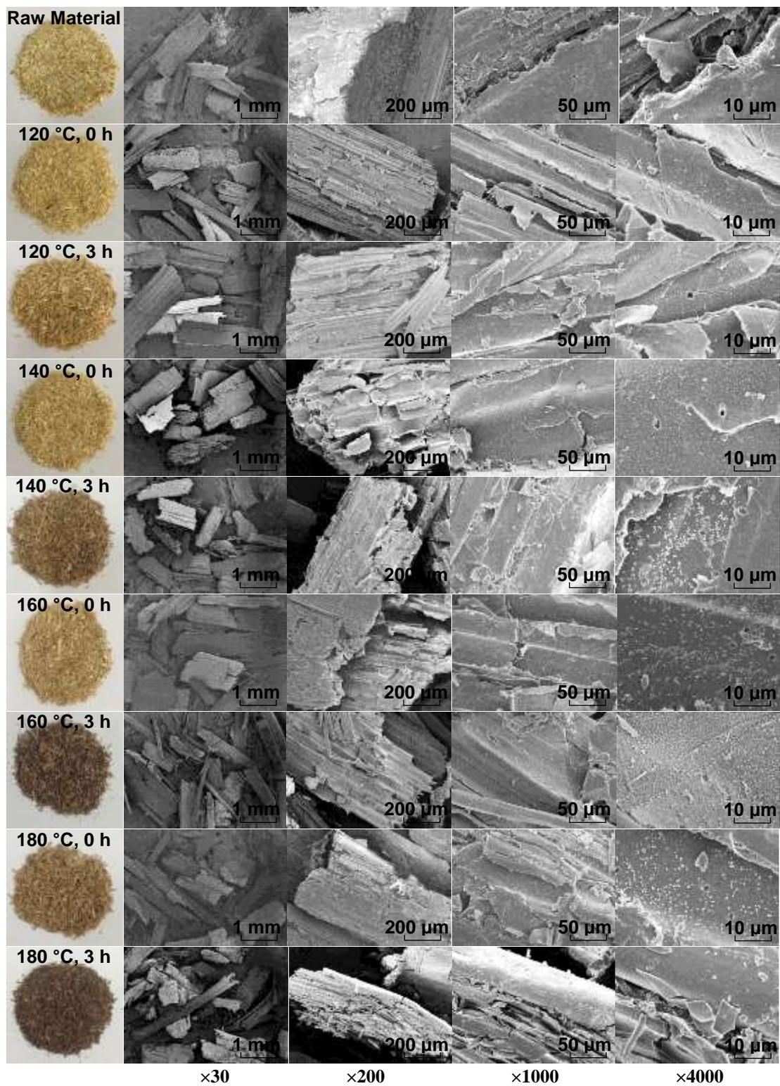
**Fig. 1.** SEM images of the raw and hydrothermally treated wheat straw with increasing temperatures and incubation periods
