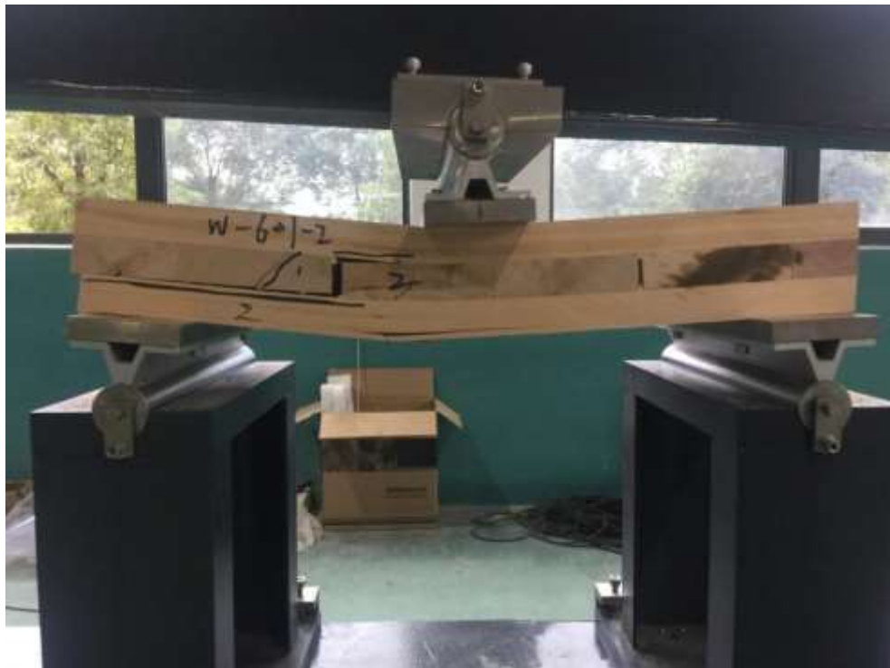
Fig. 4. Destruction surface of three-layer CLT short-span beam under three-point bending load
