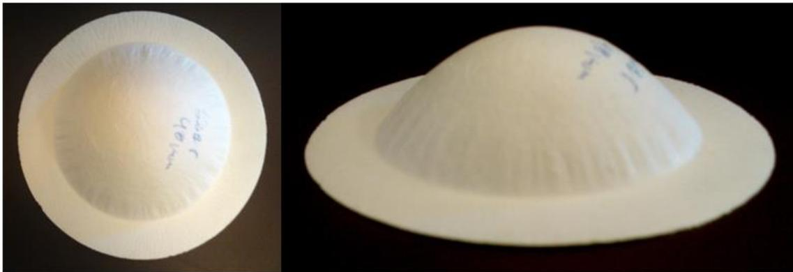
**Fig. 10.** Examples of the 3D shapes prepared with the 3D forming device at VTT, Jyväskylä; the depth of the shapes at the point of maximum curvature is approximately 21 mm (at diameter of the die of 65 mm)
