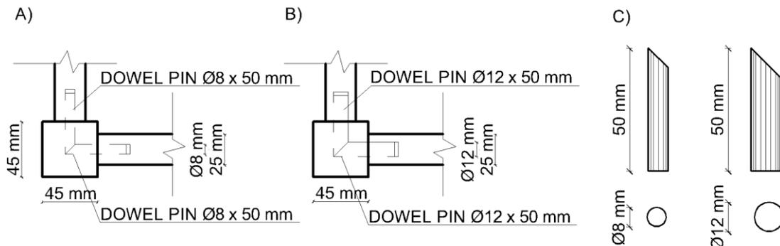
**Fig. 2.** A) Schematic depiction of the location of the dowels (C) 8 mm and 12 mm), and B) detailed view of the dowels used and their dimensions
