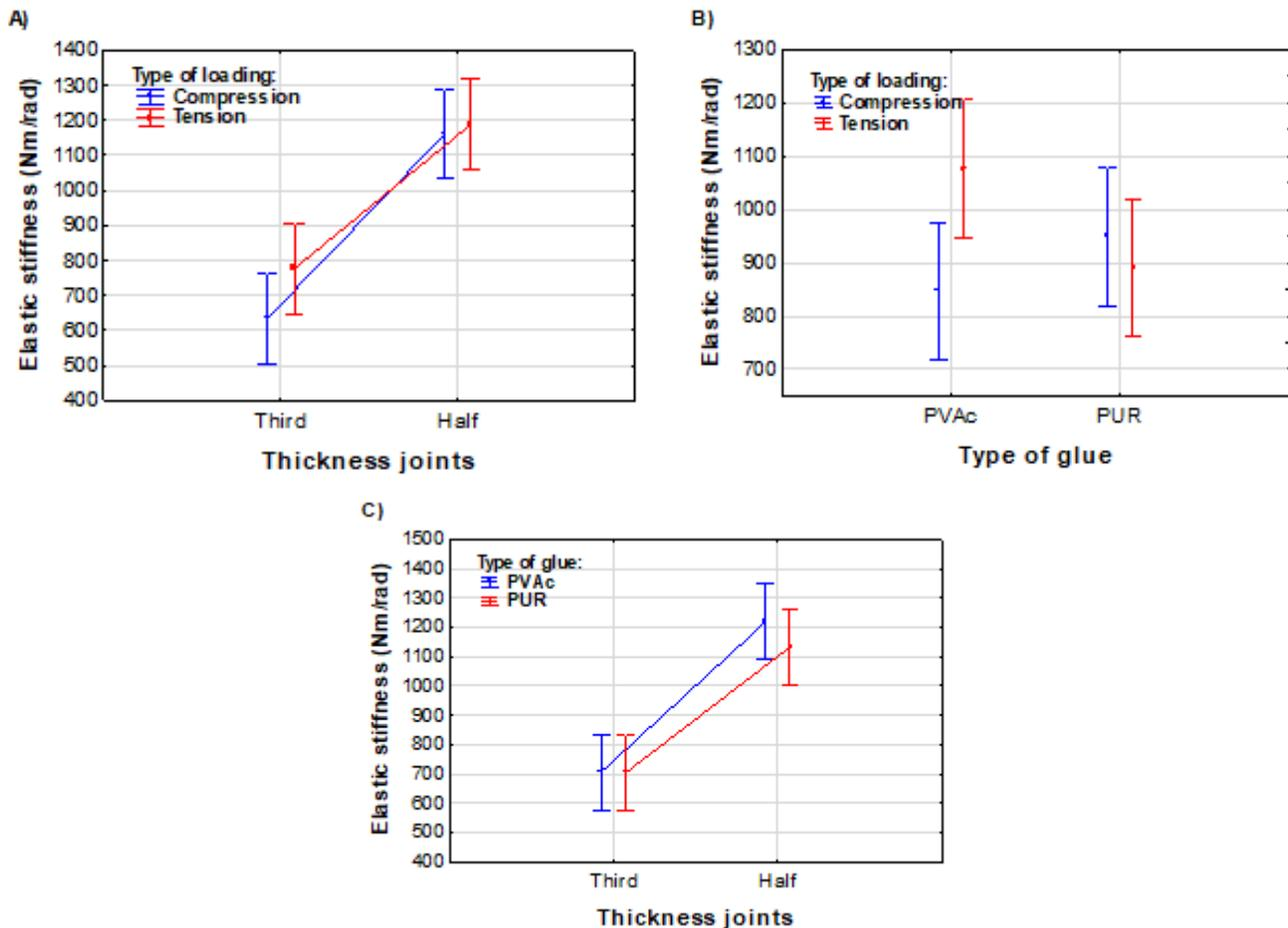
**Fig. 8.** Graphical visualization of the effect of the joint thickness and type of loading (A), type of glue and type of loading (B), and joint thickness and type of glue (C), on the elastic stiffness
