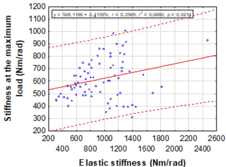
**Fig. 11.** Dependence of the stiffness at maximum load on the elastic stiffness of beech wood joints
