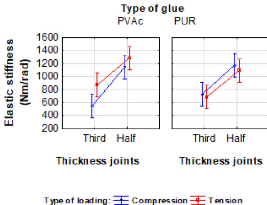
**Fig. 9.** Graphic visualization of the synergistic effect of the type of glue, thickness joints, and type of loading on elastic stiffness
