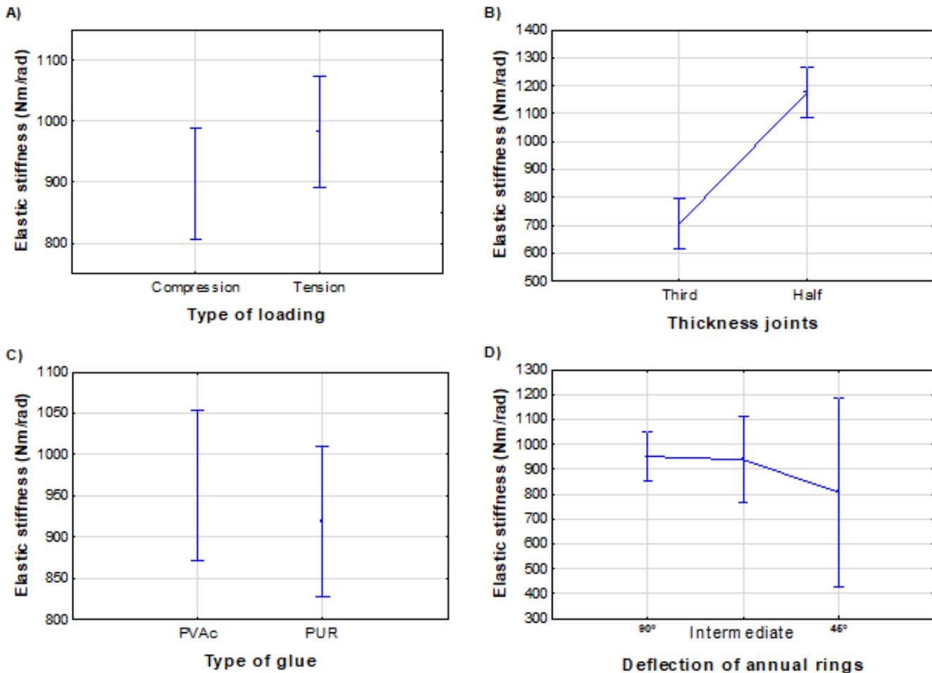
**Fig. 7.** Graphic visualization of the effect of the A) type of loading, B) joint thickness, C) type of glue, and D) deflection of annual rings on the elastic stiffness
