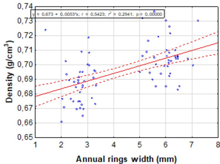
Fig. 12. Dependence of the density on the annual ring width in wood joints
