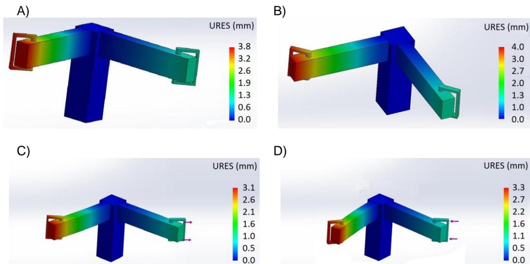
Fig. 13. A) Deformation simulation using tension loading on a joint with 8-mm dowels, B) during compression loading of a joint with 8-mm dowels, C) during tension loading of a joint with 12-mm dowels, and D) during compression loading of a joint with 12-mm dowels
