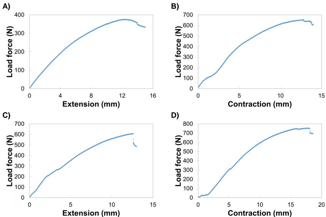
**Fig. 5.** Course of the stress-strain diagram: A) during tension loading of a joint with 8-mm dowels; B) during compression loading of a joint with 8-mm dowels; C) during tension loading of a joint with 12-mm dowels, and D) during compression loading of a joint with 12-mm dowels
