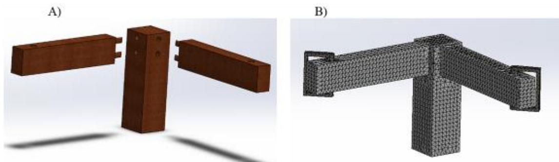
**Fig. 6.** A) Dowel joint model and B) finite element network on the model
