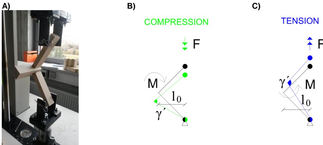
**Fig. 4.** A) Picture of the experimental while testing; B) schematic depiction of the compression loading; C) schematic depiction of the tension loading (where the original shape is depicted in black and the deformed shape is depicted in blue and green)
