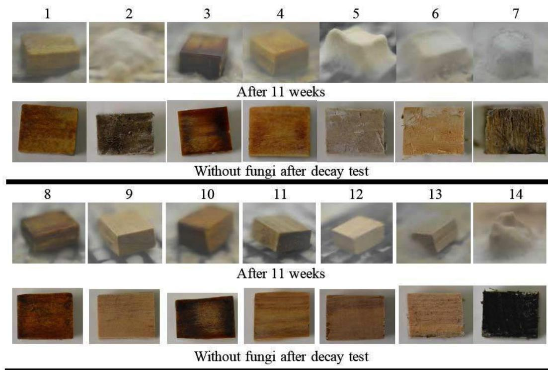
**Fig. 2.** Images of specimens in culture bottles after 11 weeks incubation, and specimens without fungi after 12 weeks decay testing
