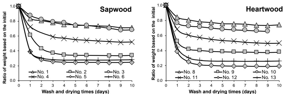
**Fig. 1.** Decrease in specimen weight after ten wash and dry cycles; each weight is given as the ratio of weights before and after leaching tests.
