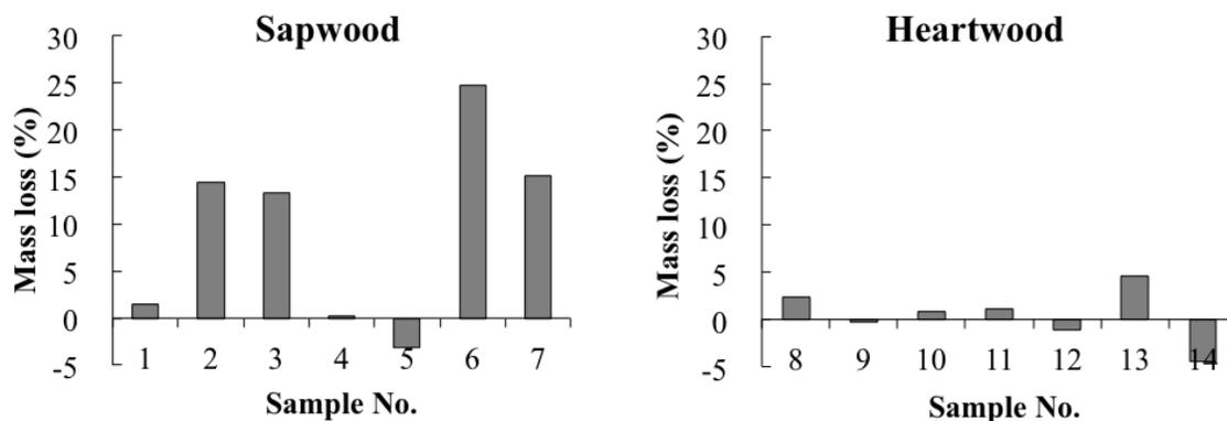
**Fig. 3.** Mass loss of specimens after twelve weeks decay testing with brown rot fungi *Fomitopsis palustris*
