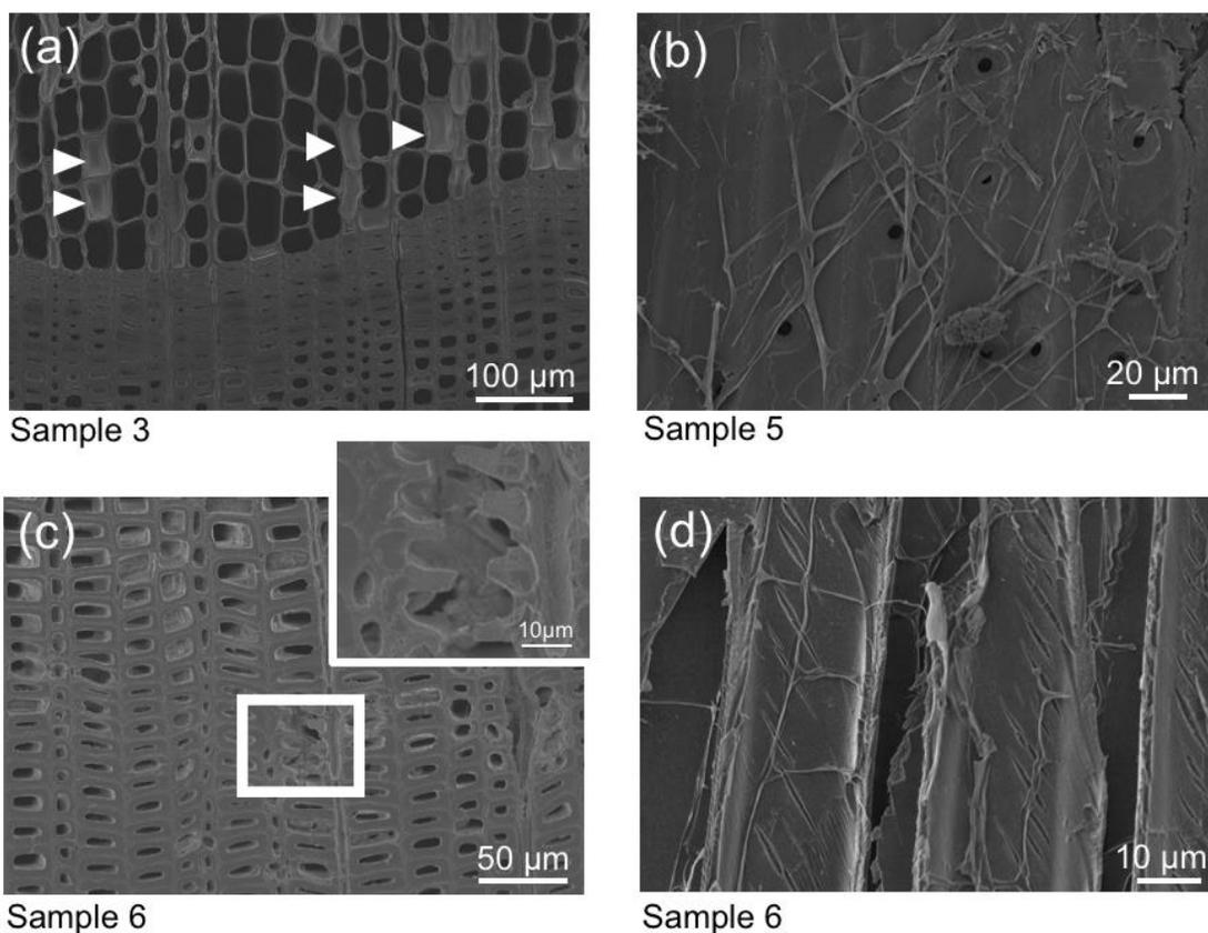
**Fig. 4.** SEM images of inner wood surfaces, transverse surface inside sample 3 (a), radial surface inside sample 5 (b), transverse surface inside sample 6 (c), and radial surface inside sample 6 (d); the arrowheads show the substances that appear like [BuVylm]I.
