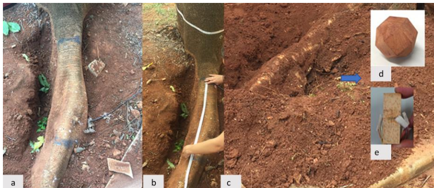
Fig. 1. Illustration of the root segment (a) and the measurement (b), root excavation for the removal process (c) to obtain ultrasonic (polyhedral, d) and static parallel (prismatic, e) specimens
