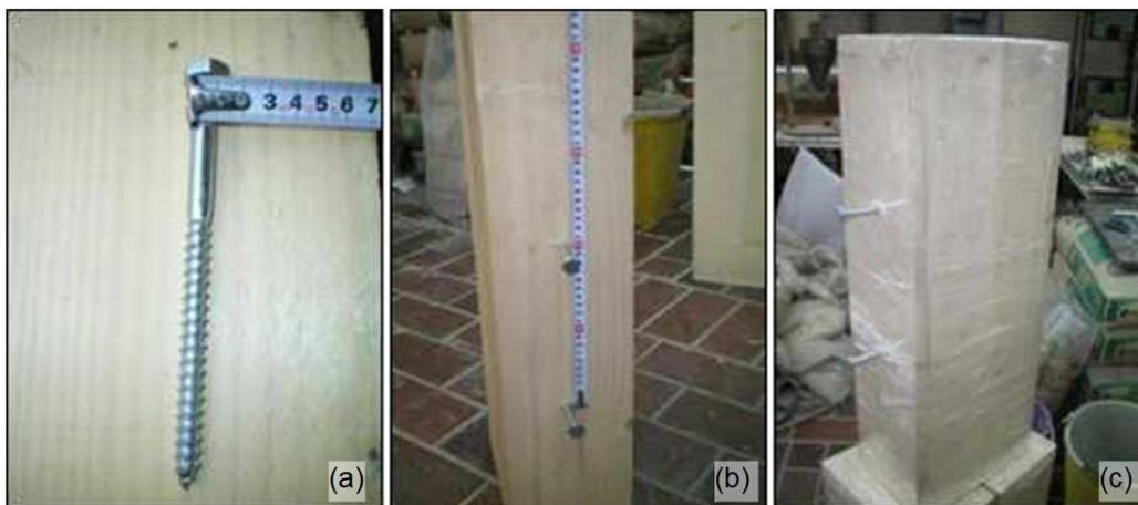
**Fig. 1.** (a) Lag screw used for slip modulus testing/evaluation; (b) spacing of the screws; and (c) timber beam covered with PVC foil
