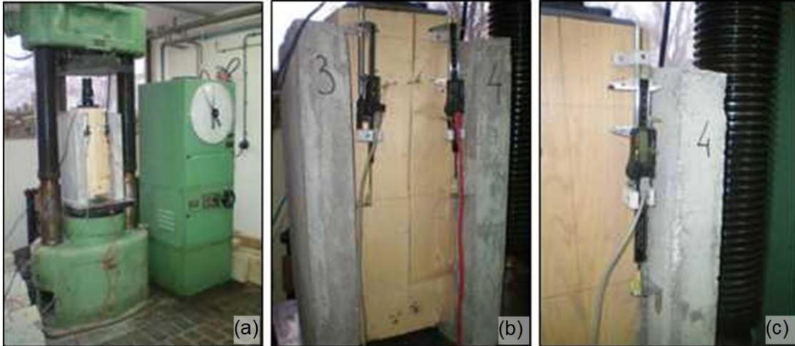
**Fig. 4.** (a) Sample during testing and (b and c) position of the calipers relative to the sample
