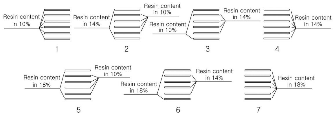
**Fig. 1.** Assembly design for LBB before hot-pressing
