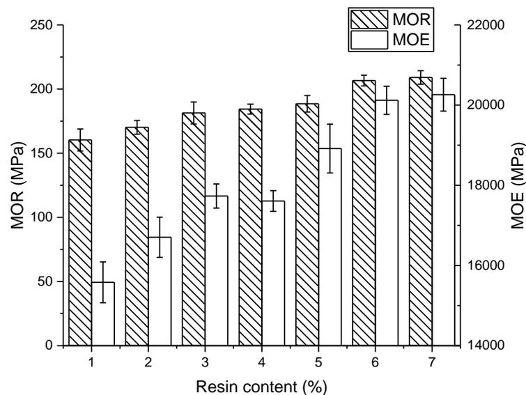
**Fig. 2.** MOR and MOE of BFRC. The resin content in the numbered columns is as follows: 1) 10% (all layers); 2) 10% and 14% (face and core); 3) 14% and 10% (face and core); 4) 14% (all layers); 5) 18% and 10% (face and core); 6) 18% and 14% (face and core); 7) 18% (all layers).
