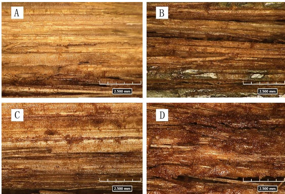
**Fig. 6.** (A) The bundles were examined *via* 3D digital microscope for the resin content of 10%. (B) The bundle was impregnated with resin of a high solid content and a resin content of 18%. (C) The bundle was impregnated with resin with a resin content of 14%. (D) The bundle was impregnated with raw resin with a solid content of 45.7% and a resin content of 14%.
