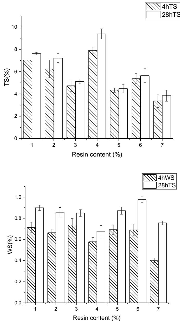
**Fig. 4.** TS and WS of BFRC. The resin content in the numbered columns is as follows: 1) 10% (all layers); 2) 10% and 14% (face and core); 3) 14% and 10% (face and core); 4) 14% (all layers); 5) 18% and 10% (face and core); 6) 18% and 14% (face and core); 7) 18% (all layers)
