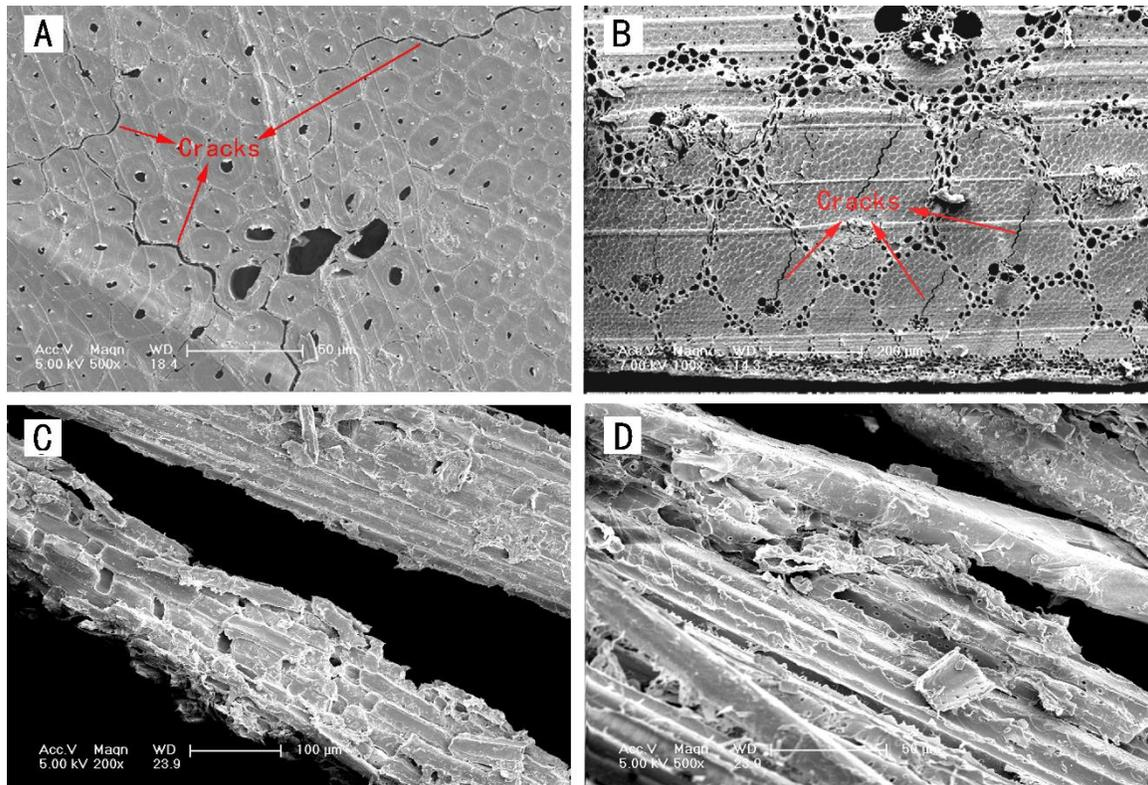
**Fig. 5.** (A) (B) SEM images of LBB after mechanical roll-pressing treatment: The fiber bundle is composed of several elementary fibers observed in the radial section. (C) (D) SEM images of bamboo showing the roughness of the fiber bundles after mechanical pressing observed in the transverse section.
