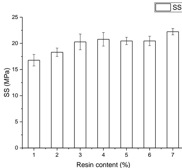
**Fig. 3.** SS of BFRC. The resin content in the numbered columns is as follows: 1) 10% (all layers); 2) 10% and 14% (face and core); 3) 14% and 10% (face and core); 4) 14% (all layers); 5) 18% and 10% (face and core); 6) 18% and 14% (face and core); 7) 18% (all layers).
