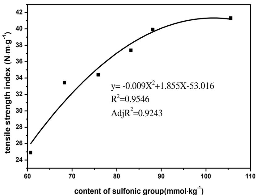
Fig. 2. Effect of content of sulfonic group content on tensile strength index
