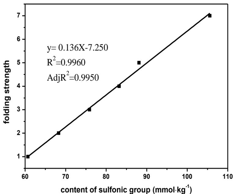
Fig. 3. Effect of content of sulfonic group content on folding strength
