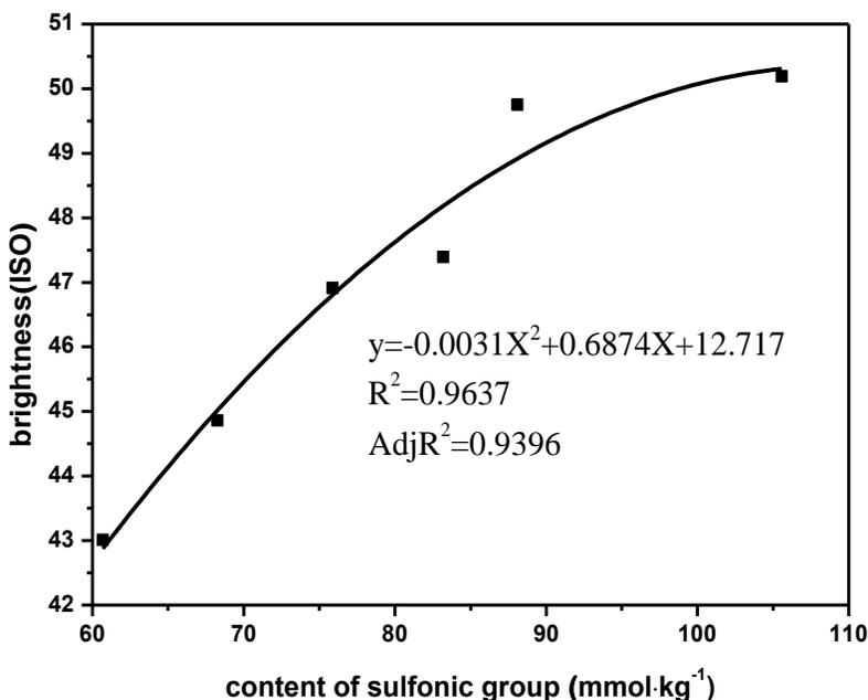
Fig. 1. Effect of sulfonic group on brightness
