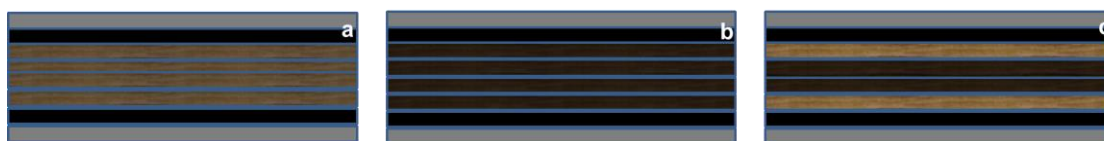
Fig. 3. Schematic of 2/1 layup of the fabricated FML a) CFC, b) CSC, and c) CFSSFC
