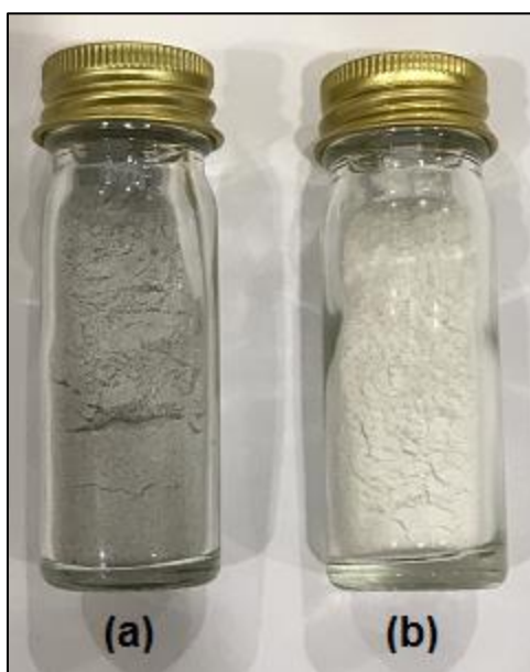
Fig. 2. Appearance of RHS samples: (a) RHS extracted from untreated rice husks calcined at 700 °C; and (b) RHS extracted from solvent-thermal treated and leached rice husks in 1.0 M HCl, followed by calcination at 700 °C
