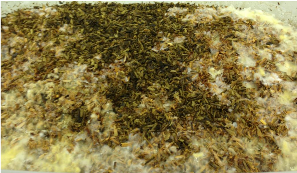
Fig. 5. F. radiculosa growing on copper-treated wood for 35 days (Akgul 2016)
