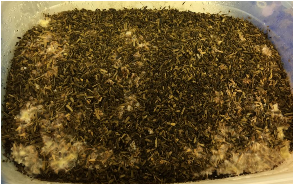
Fig. 4. F. radiculosa actively growing on copper-treated wood for 25 days (Akgul 2016)
