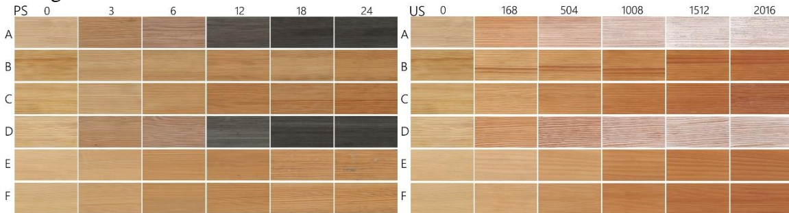
Fig. 5. The scans of coating systems (A-F) during natural weathering NW (0 months, 3 months, 6 months, 9 months, 12 months, 18 months, and 24 months) on the left and artificial weathering AW (0 h, 168 h, 504 h, 1008 h, 1512 h, and 2016 h) on the right, with the evaluation based on EN ISO 4628 (2003)
