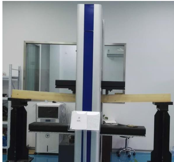
Fig. 1. Four-point bending test of glulam
