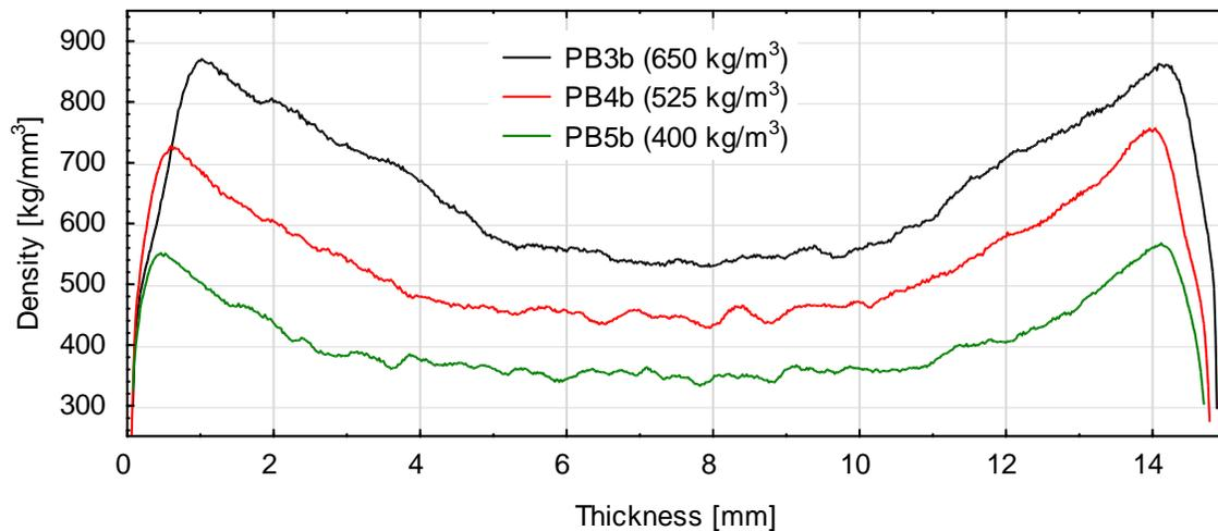
**Fig. 3.** Density profiles of boards pressed in an automatic cycle
