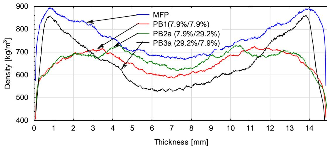
Fig. 1. Density profiles of industrial MFP and laboratory boards with density of 650 kg/m<sup>3</sup>
