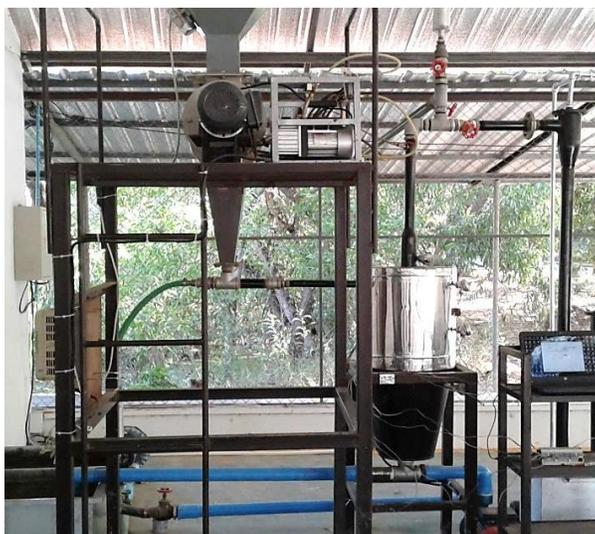
Fig. 3. Photograph of biomass cyclone gasifier system
