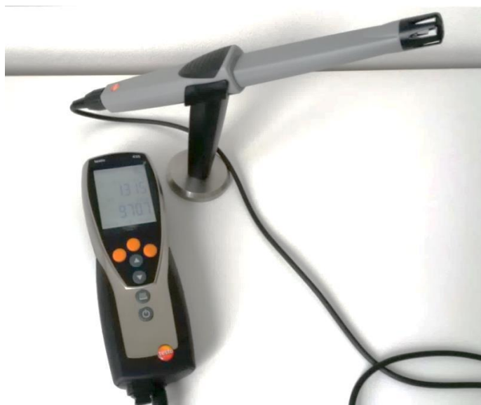
Fig. 1. Testo 435 – 2 measuring instrument with IAQ probe
