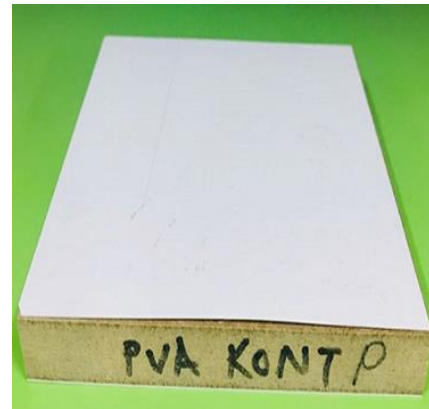
Fig. 12. Control sample: PCV veneer bonded with PVAc adhesive
