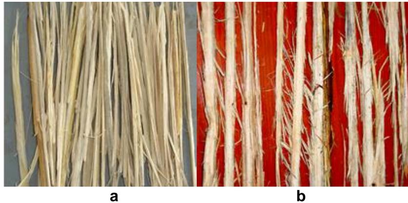
**Fig. 3.** Geometric shapes of the wood bundle sticks produced via the combing process in different directions: (a) combed with the grain and (b) combed against the grain
