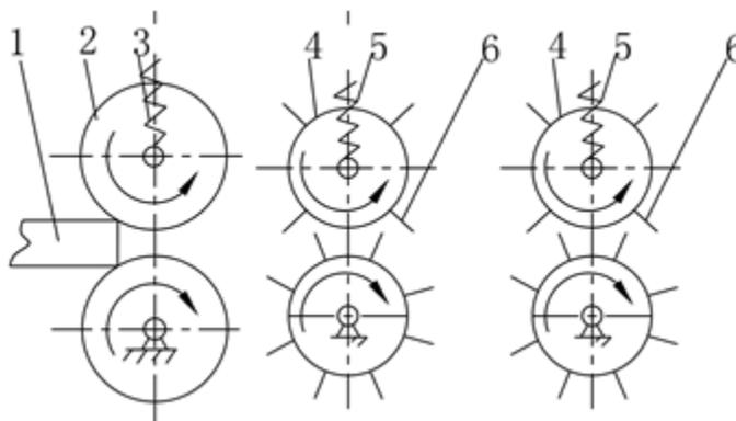
**Fig. 2.** Structural schematic diagram and running mechanism of the combing equipment: (1) feedstock (sawmill slabs residue), (2) compression rollers, (3) and (5) spring controllers; (4) combing rollers, and (6) combing knives
