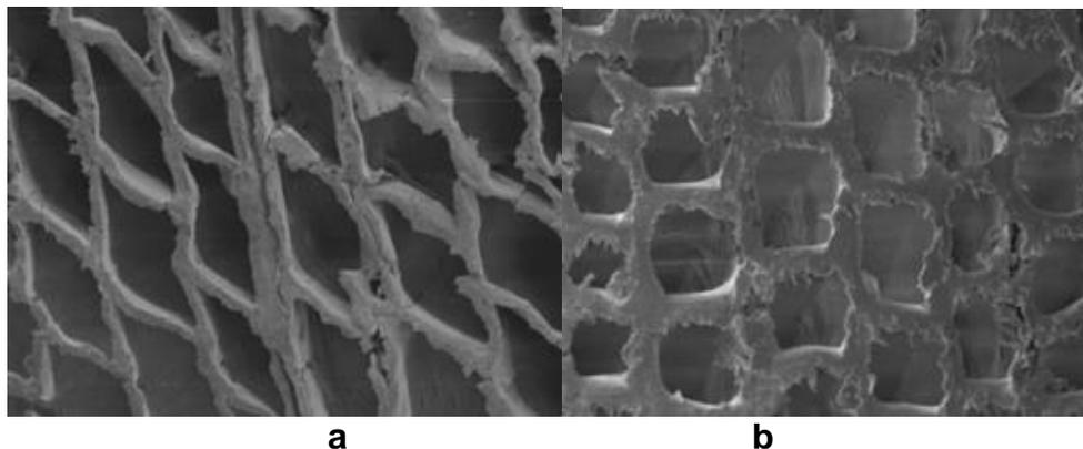
**Fig. 4.** Cellular structures of the wood sticks at two different MCs: (a) 15.3% and (b) 35.7%
