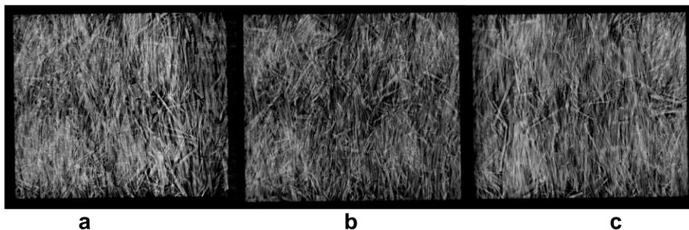
**Fig. 9.** CT chart of the horizontal faults of the scrimber: (a) surface layer, (b) core layer, and (c) bottom layer
