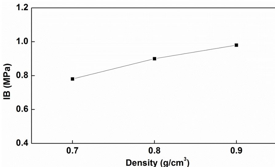
Fig. 8. Relationship between the density and IB
