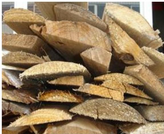
**Fig. 1.** Appearance of the Chinese fir sawmill slabs
