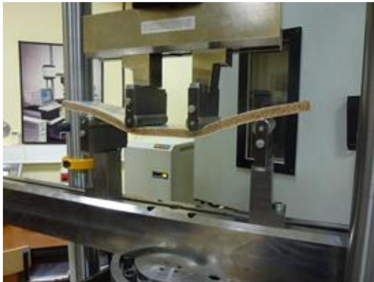
**Fig. 3.** Static four-point bending tests performed on 15-mm-thick Plycork Al
