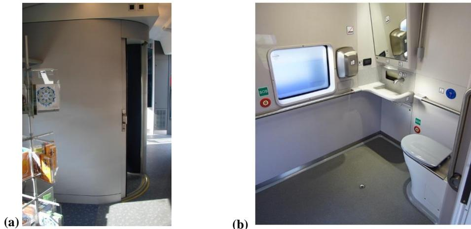
**Fig. 16.** Application of Plycork Al composite in the train toilet: (a) door and (b) floor and walls
