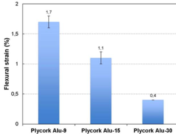
Fig. 7. Flexural strain of Plycork Al composites with thicknesses of 9 mm, 15 mm, and 30 mm
