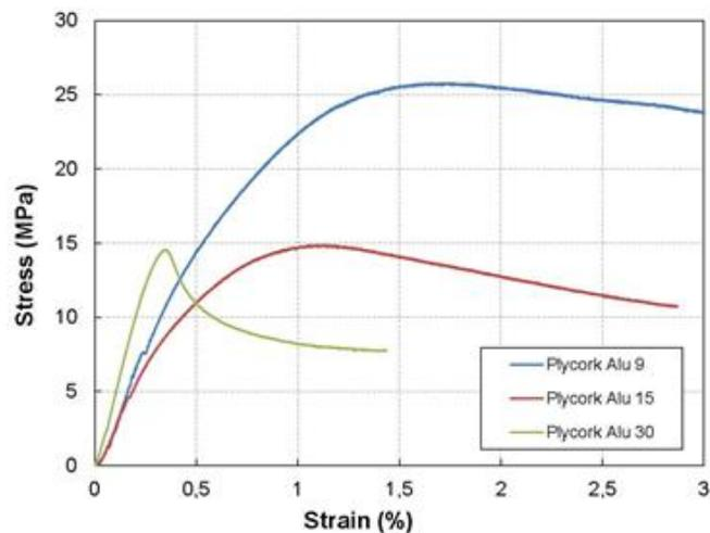
**Fig. 5.** Bending stress as a function of strain of Plycork Al composites with thicknesses of 9 mm, 15 mm, and 30 mm
