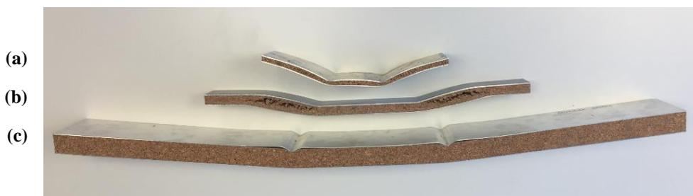
**Fig. 11.** Samples of Plycork Al composites with thicknesses of (a) 9 mm, (b) 15 mm, and (c) 30 mm after the four-point bending tests
