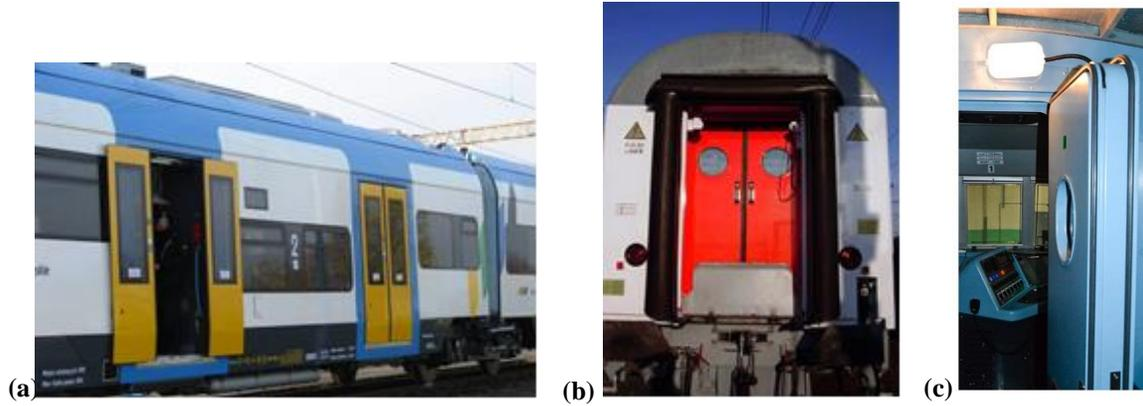
**Fig. 14.** Application of a Plycork Al composite in (a) the entrance door of the train, (b) the partition door of the train, and (c) the door of the train engine
