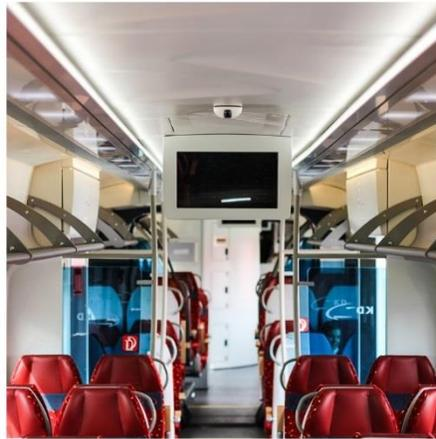
**Fig. 17.** Application of Plycork Al composite in luggage racks on the train
