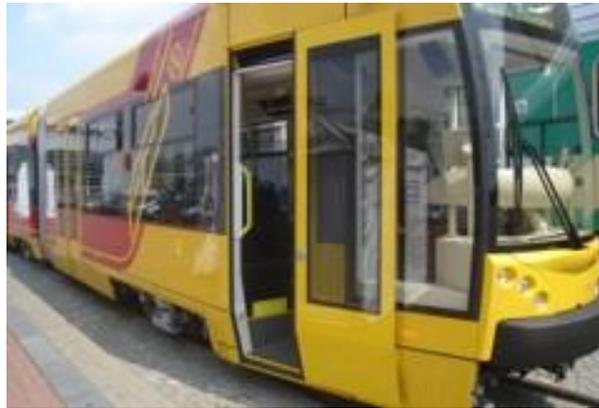
**Fig. 15.** Application of Plycork Al composite in the entrance door of the tram
