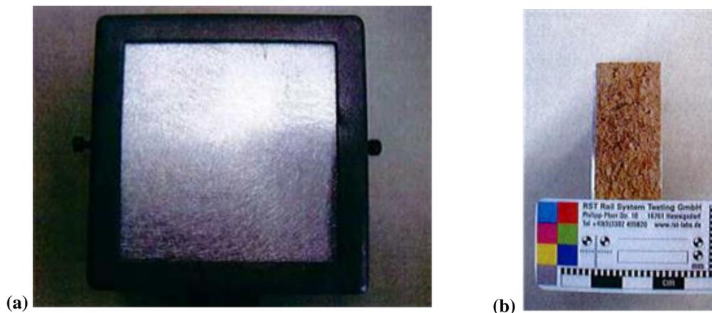
**Fig. 4.** Plycork Al 42-mm-thick sample before the test: (a) front face and (b) sideways
