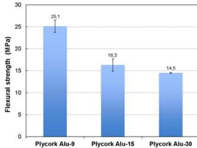
Fig. 6. Flexural strength of Plycork Al composites with thicknesses of 9 mm, 15 mm, and 30 mm
