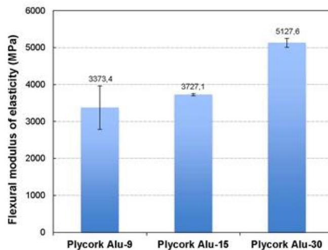
Fig. 8. Flexural modulus of elasticity of Plycork Al composites with thicknesses of 9 mm, 15 mm, and 30 mm
