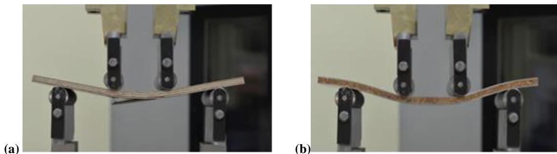
**Fig. 9.** Four-point bending test for (a) 9-mm-thick birch plywood panel (b) 9-mm-thick Plycork Al
