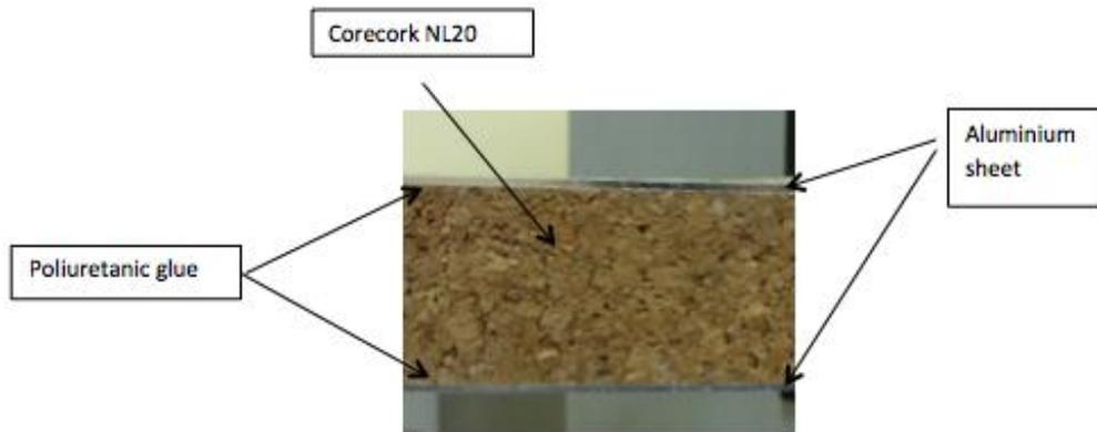
Fig. 1. 30-mm-thick Plycork Al composite
