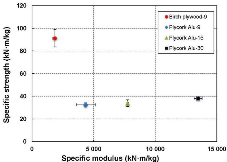
**Fig. 12.** Specific flexural strength and specific modulus of elasticity of Plycork Al composites with thicknesses of 9 mm, 15 mm, 30 mm compared to birch plywood of 9 mm
