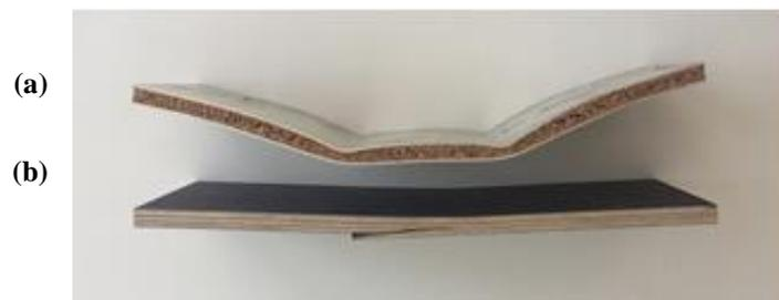
**Fig. 10.** Samples of 9-mm-thick: (a) Plycork Al composite and (b) birch plywood after the four-point bending tests
