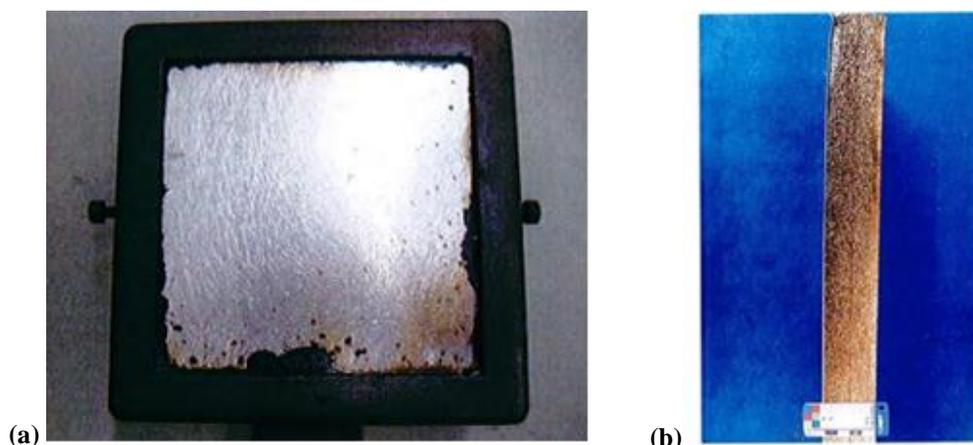
**Fig. 13.** Plycork Al samples after the fire resistance test: (a) front face, (b) sideways
