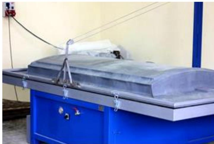
**Fig. 2.** Membrane vacuum press
