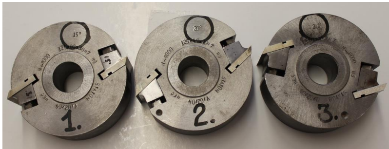
Fig. 2. Milling cutters with rake angles of 15° (1), 20° (2), and 30° (3)
