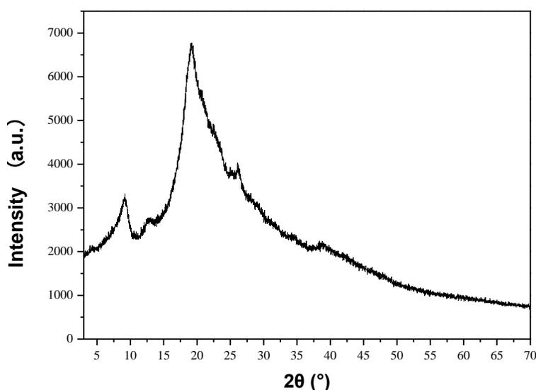
**Fig. 3.** XRD patterns of the polyuronic acid
