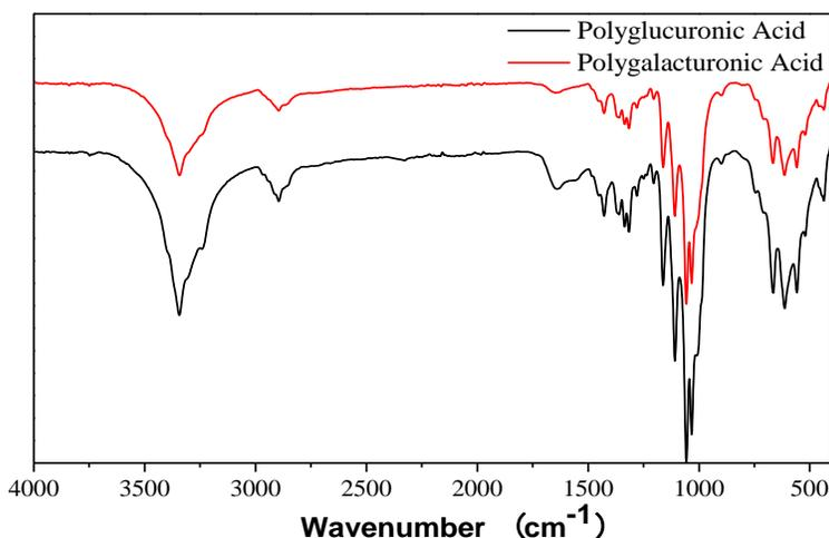
**Fig. 1.** FTIR spectra of the polyuronic acids
