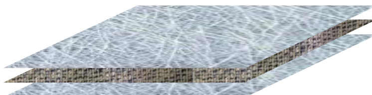
Fig. 1. Structural layout of hybrid glass/kenaf configuration
