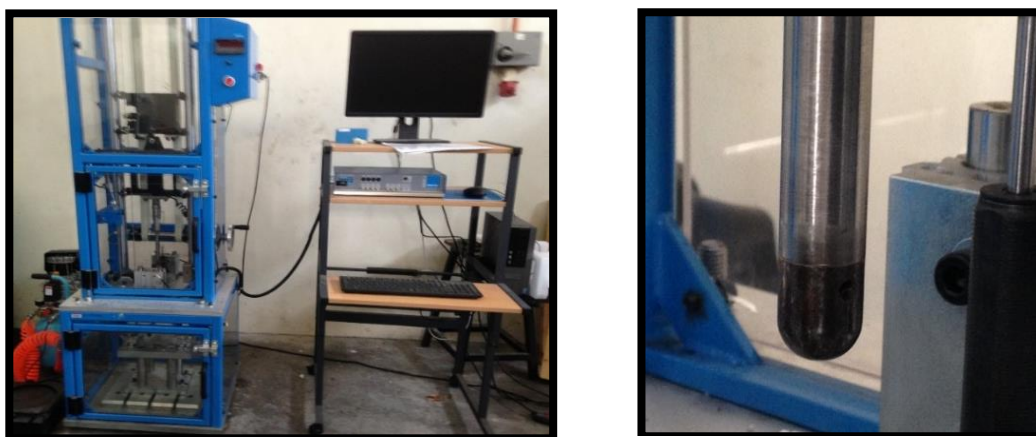
Fig. 2. Instrumented Drop Weight Impact tester with tup
