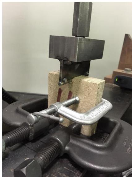
**Fig. 6.** Test setup for evaluating half-hole screw-bearing strength properties in particleboard
