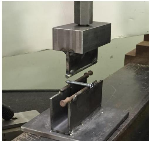
**Fig. 7.** Setup for evaluating the bending moment capacity of screws
