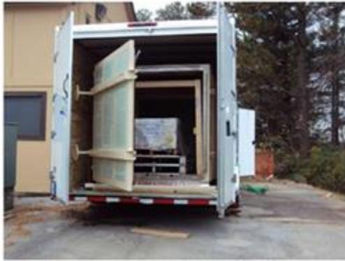
**Fig. 4.** Vacuum steam chamber used in the tests
