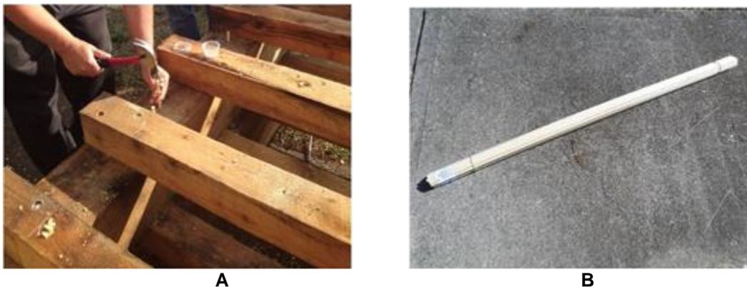
Fig. 6. The 0.48 cm (3/8 inches) hole was drilled (A) and tightly plugged with the dowels (B) after the larva was inserted
