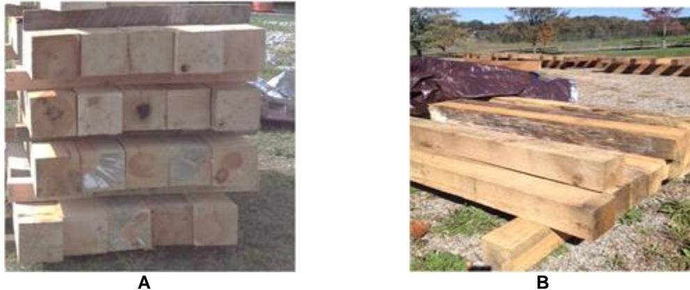
**Fig. 1.** The 20.32 cm × 20.32 cm large timbers (A) and the 10.16 cm × 10.16 cm deck timbers (B) of southern pine, yellow-poplar, and oak spp.
