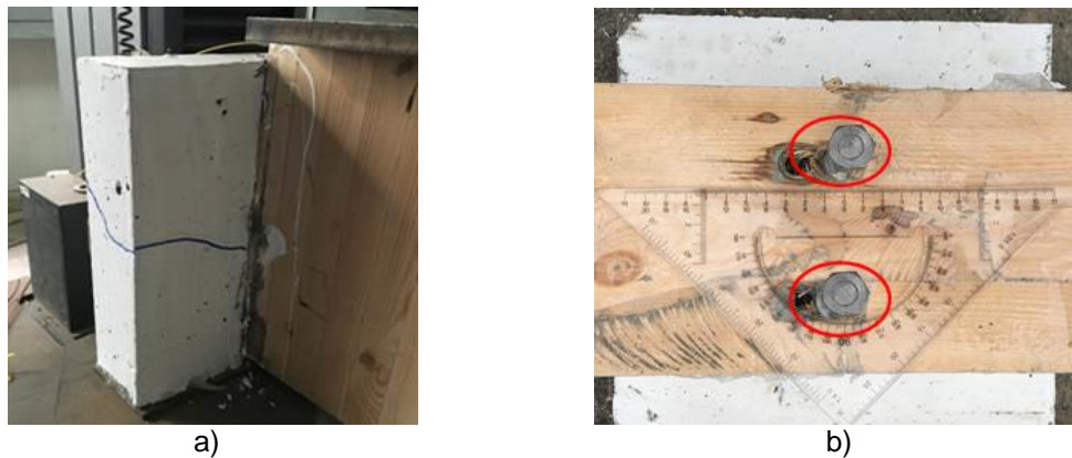
Fig. 5. Test phenomena and failure mode of push-out specimens: a) horizontal crack on the concrete slab, and b) compressive deformation of the glulam and bending deformation of the lag screw
