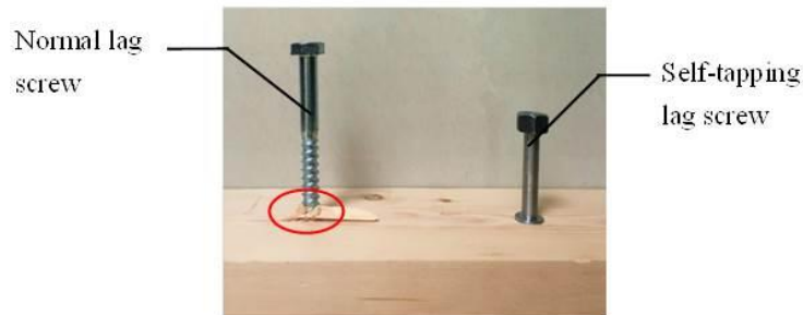
Fig. 1. Comparison between the normal lag screw and self-tapping lag screw
