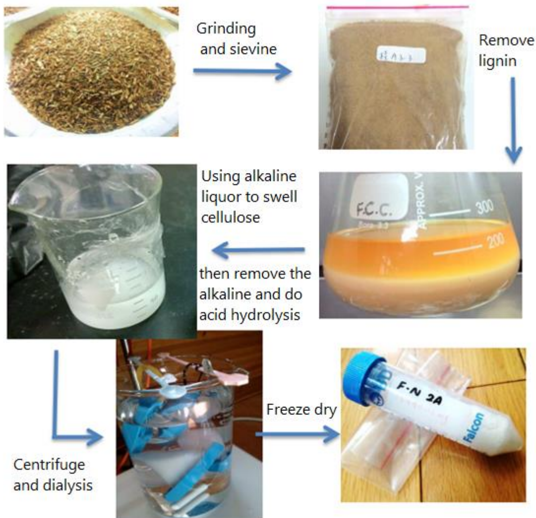
Fig. 1. Processing procedures for BCNW
