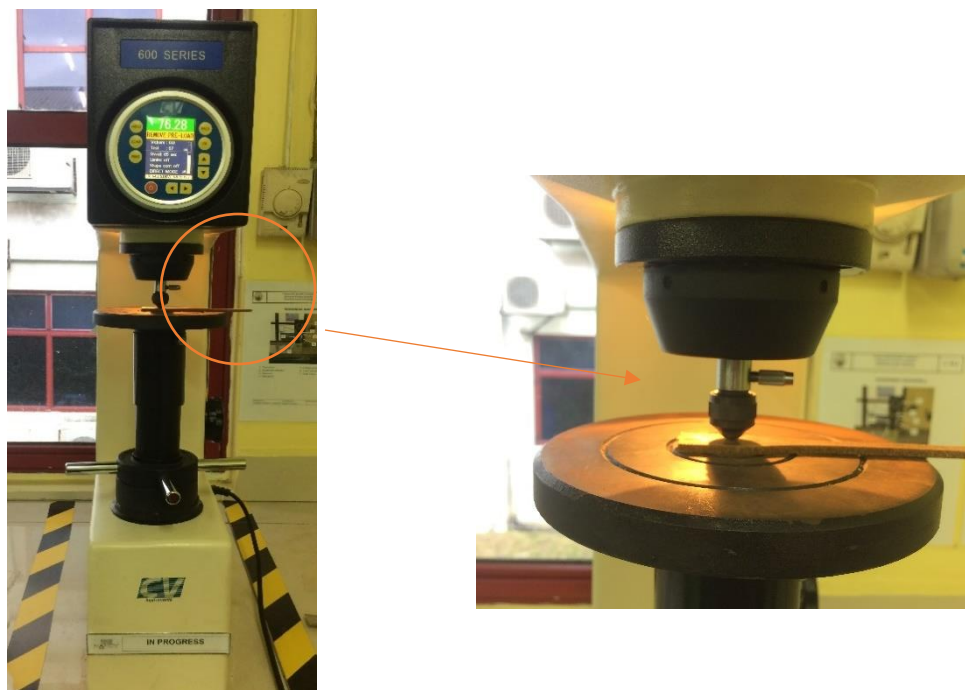
Fig. 4. The specimen placed on the Rockwell hardness machine
