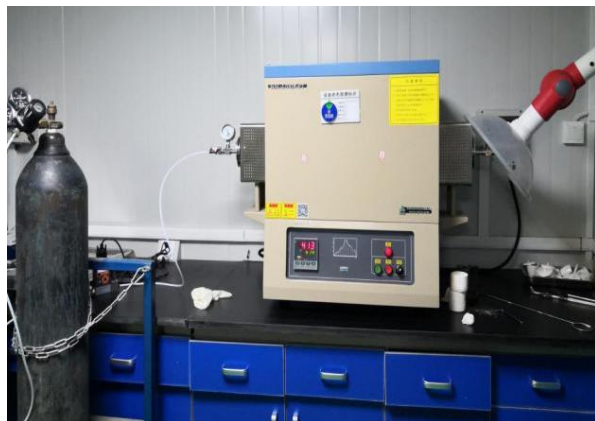
Fig. 2. Horizontal fixed tubular furnace
