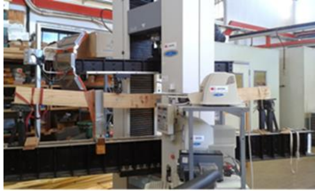
Fig. 3. Static four-point bending test set up
