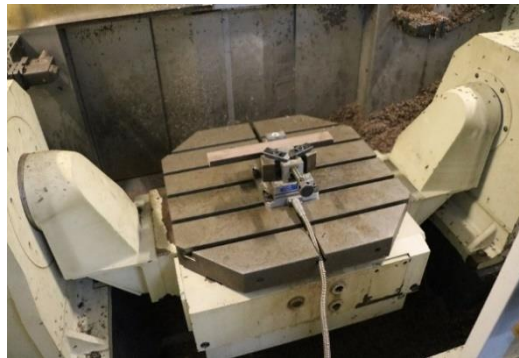
Fig. 2. Kistler 9257B three-way dynamometer installed on the machine
