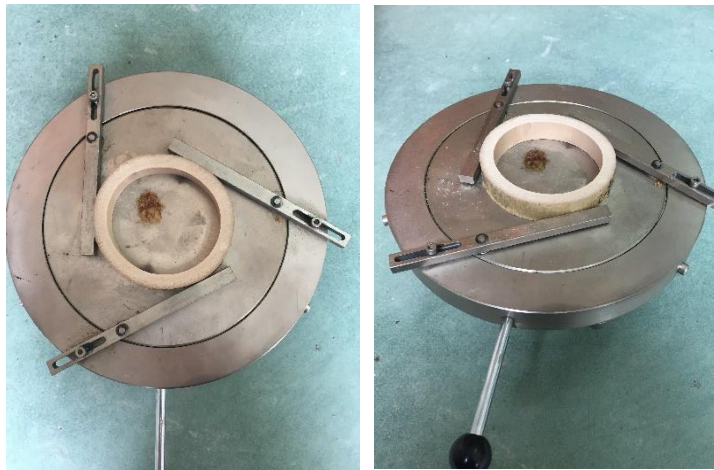
Fig. 5. Centering device of the specimen
