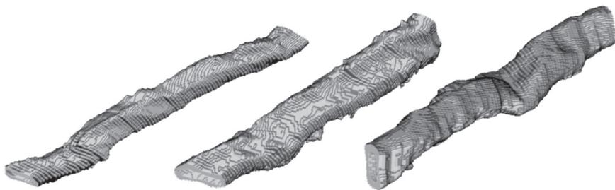
**Figure 2.** Examples of isolated fibers segmented from a XR- $\mu$ CT representation of a fibrous structure [24].
