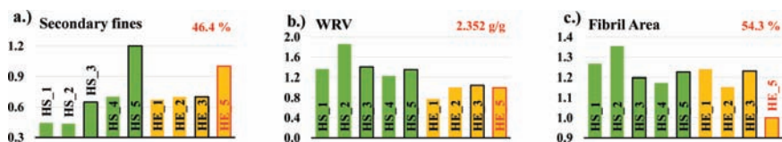
Figure 7. Trial setup for evaluation of the influence of secondary fines quality and quantity: Characterization of separated fines fractions of fines obtained by the variation of refiner settings: (a) secondary fines content; (b) WRV; (c) fibril area.
