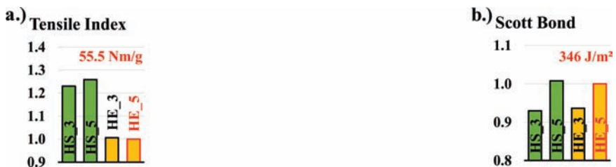
Appendix 2. Development of strength properties as a result of changing fibre quality: (a) Tensile Index, (b) Scott Bond.
