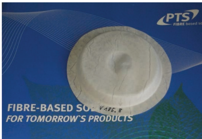
Figure 15. Thermoformed cup made of DA1-3 dialcohol cellulose sheet.
