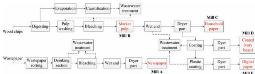
Figure 2. Process schematics of five pulp and paper mills.
