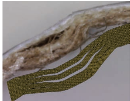
Figure 37. Experimental and numerical work from [71]. (a) Creasing result for Paperboard A–C. (b) Folding curves at different crease depths for paperboard A in MD, (c) Comparison of FEM model and experimental bending deformation at 20-degree bend for Paperboard A in MD for board creased to d = 0.0 mm.
