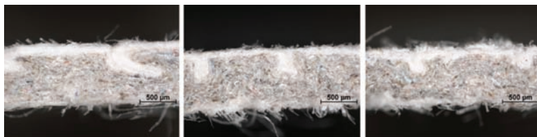
Figure 39. Cross-sectional cut of walls made by deep-drawing at different blank holder forces in microscopic scale. Picture reproduced with kind permission of Dr. M. Hauptmann, TU Dresden.
