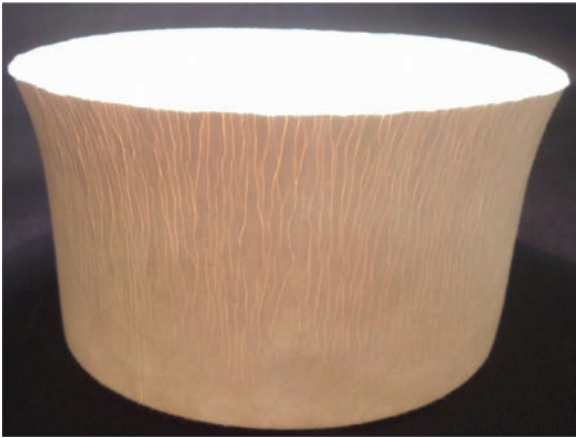
Figure 28. Formed shape with wrinkles and microscope image of the wrinkles.
