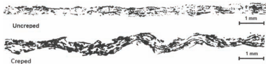
Figure 84. Cross-sectional images of uncreped and creped paper, [96].
