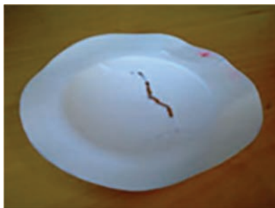
Figure 21. Typical mode of rupture in paperboard hydroforming. Fracture occur perpendicular to the weakest material direction, [39].
