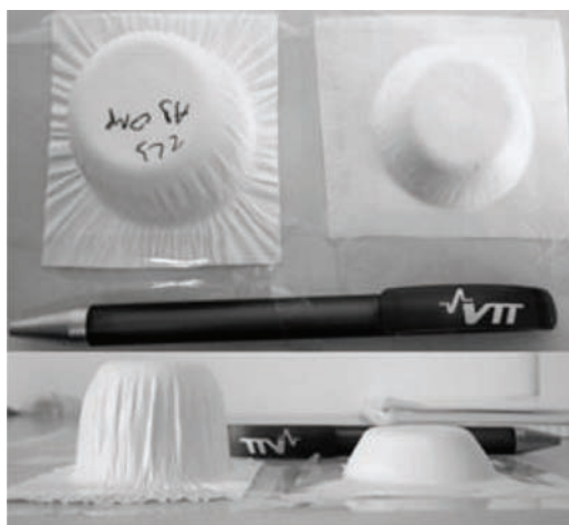
Figure 91. Examples of the shapes fabricated from the 200 g/m 2 extensible paper formed in the sliding ( left ) and fixed ( right ) blank processes, [105].
