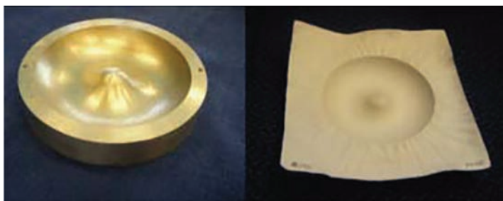
Figure 87. Forming cavity (nominal stretch 1.21) and formed bleached softwood kraft pulp sheet with 20% polylactide latex, [71].
