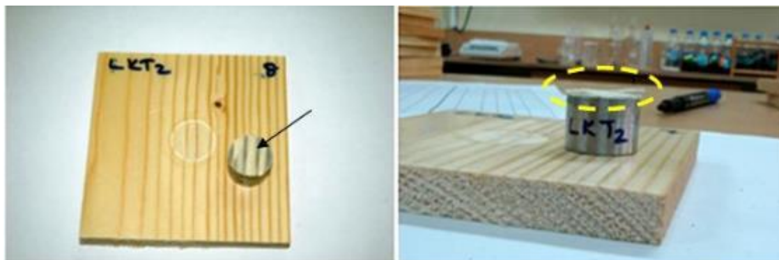
Fig. 10. Breakage from the spruce samples after adhesion strength experiment
