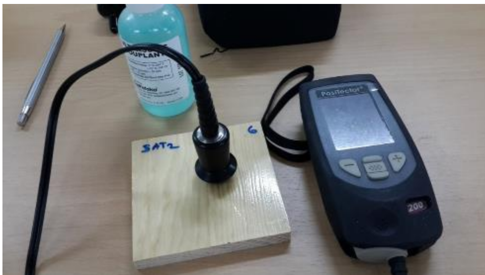
Fig. 4. Determining dry film thickness
