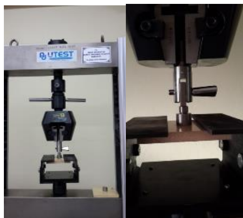
Fig. 8. Cutting the pull-off test cylinder circumference to the layer
