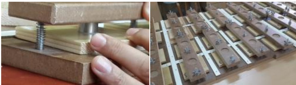
Fig. 7. Attaching the pull-off test cylinders to sample surfaces using mold
