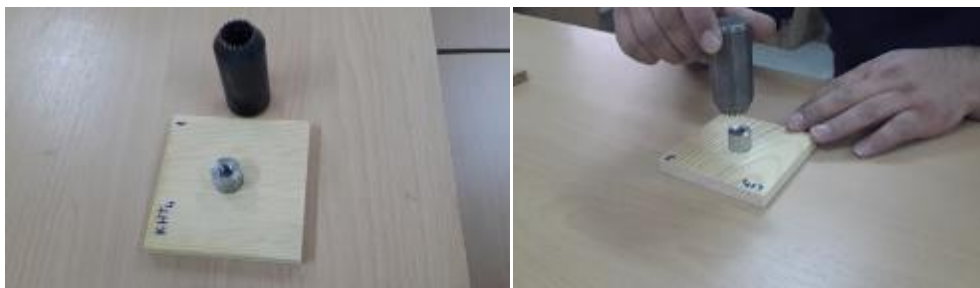
Fig. 8. Cutting the pull-off test cylinder circumference to the layer
