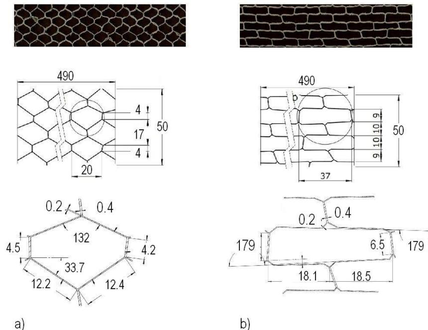
**Fig. 2.** Core section and dimensions of a) hexagonal and b) rectangular cell (dimensions in mm)
