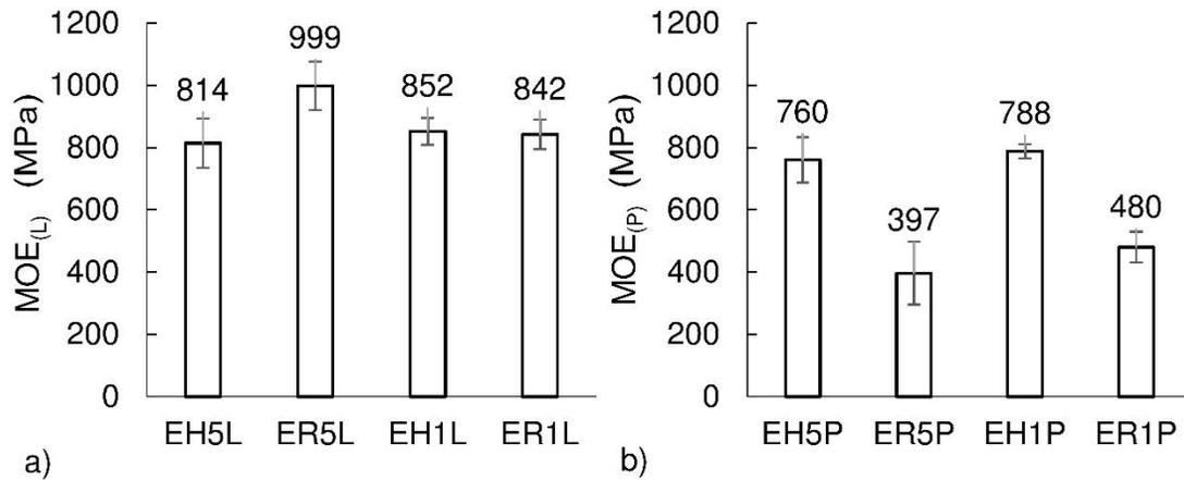
**Fig. 6.** Modulus of elasticity of the honeycomb panels for direction: a) (L) and b) (P)
