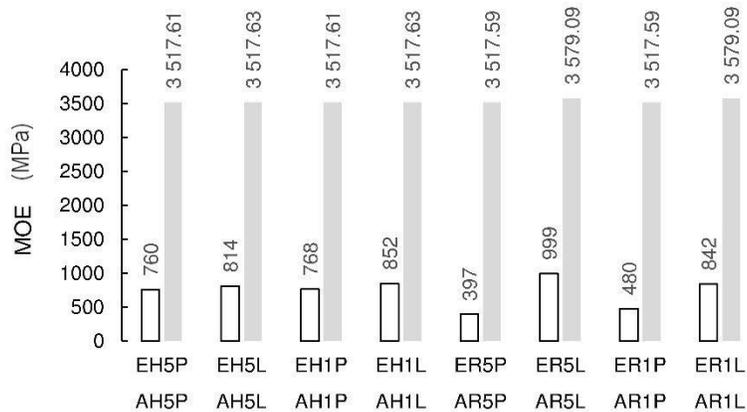
**Fig. 8.** Modulus of elasticity of honeycomb panels
