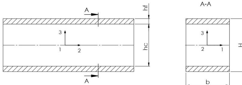
Fig. 4. Measurements of the sandwich beam
