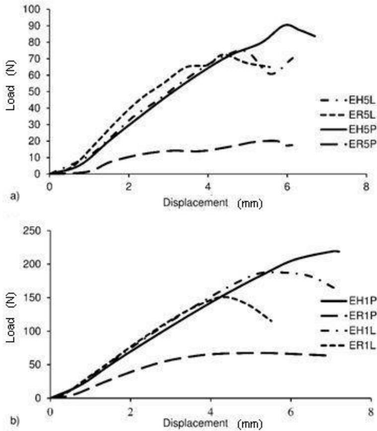
Fig. 5. Stiffness of samples: a) 50-mm-wide and b) 100-mm-wide
