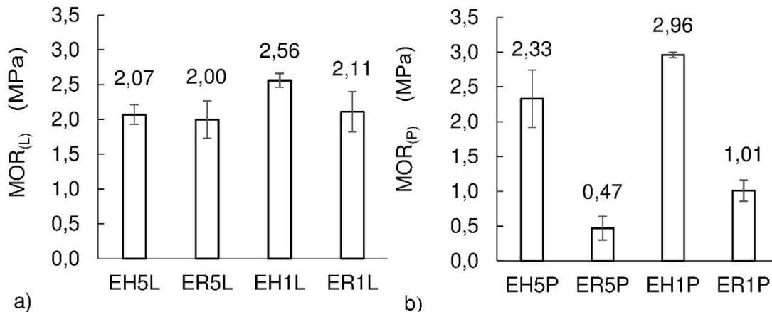
**Fig. 7.** Bending strength of the panels for direction a) (L) and b) (P)
