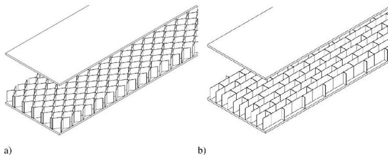
**Fig. 3.** Variants of panels prepared for tests with: a) hexagonal core and b) rectangular core
