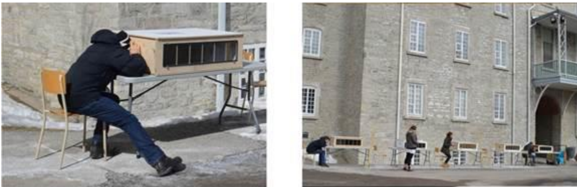
Fig. 1. Observer looking inside the model (left). Experimental settings with the five scale models aligned in the parking lot, South-East-facing, with observers (right).
