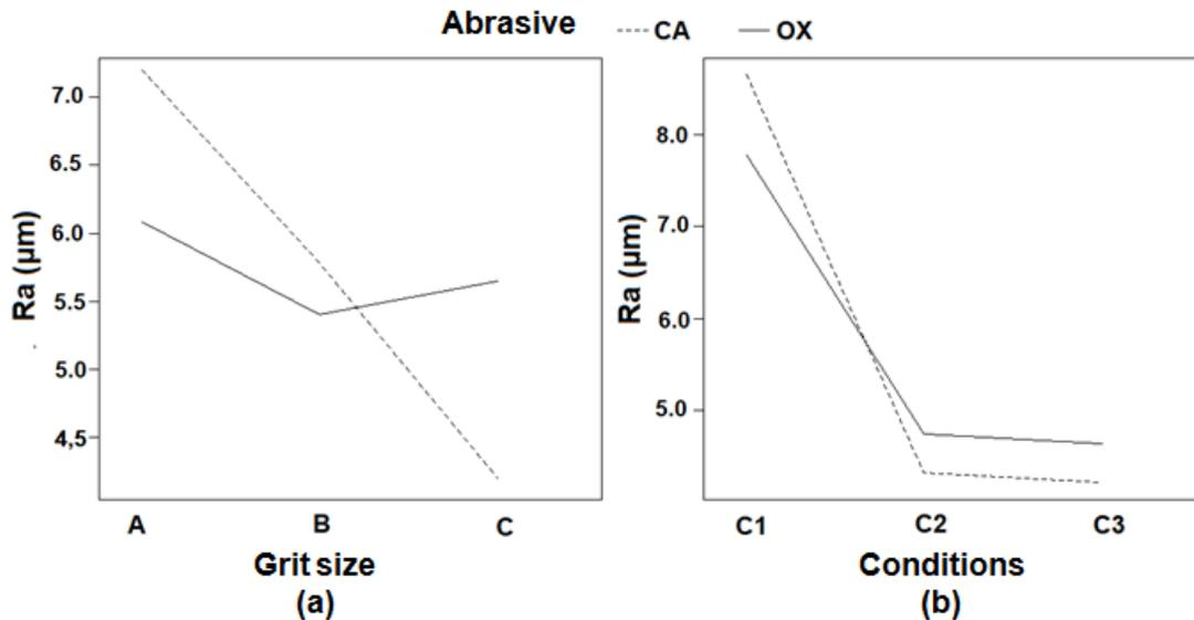
**Fig. 3.** Interaction graph in relation to the behavior of surface roughness during the parallel sanding of the wood *P. elliottii* to: (a) abrasive and grit size; (b) abrasive and condition
