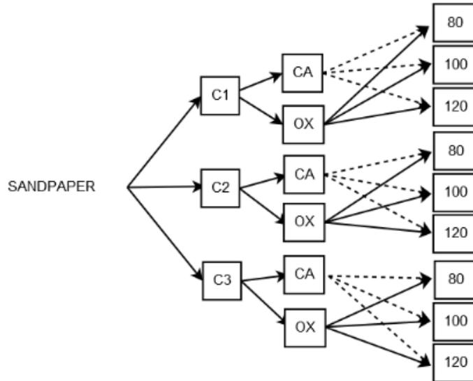
**Fig. 1.** Full factorial planning flowchart adopted for sanding tests
