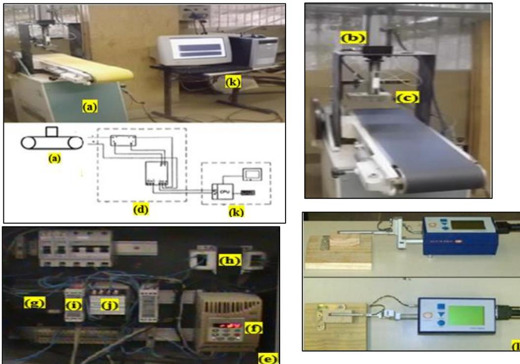
**Fig. 2.** The components of the test structure include a flat sander, monitoring system, and data acquisition, together with the roughness used in the sanding process. The diagram key is as follows: (a) Flat sander, (b) pneumatic cylinder, (c) sample fixing rod, (d) monitoring system, (e) electric panel, (f) frequency inverter, (g) power supply, (h) transformer, (i) load cell transducer, (j) current cell transducer, and (k) microcomputer with LabVIEW software installed
