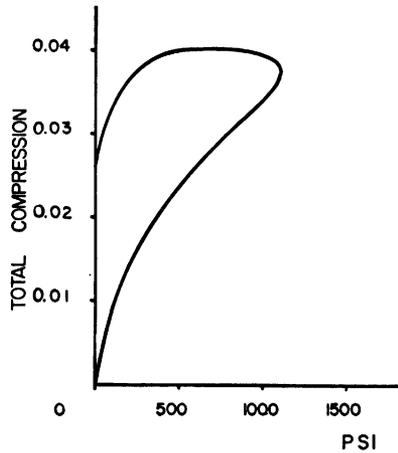
Fig. 32—Compression of newsprint packing plus a single sheet of rotogravure newsprint
