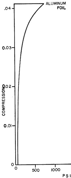
Fig. 7—Stress/strain curve for aluminium foil
