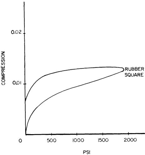
Fig. 5—Stress/strain curves for rubber cubes in compression
