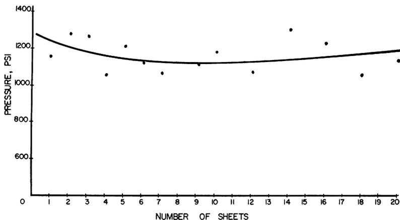
Fig. 10—Peak pressure used for different numbers of sheets tested
