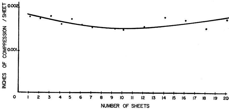
**Fig. 12**—Compression per sheet as a function of the number of sheets tested
