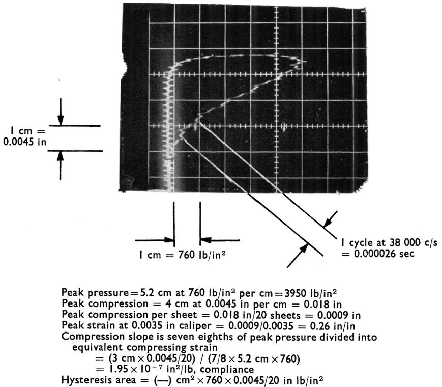
Fig. 3—Typical oscilloscope trace from the dynamic compressibility test
