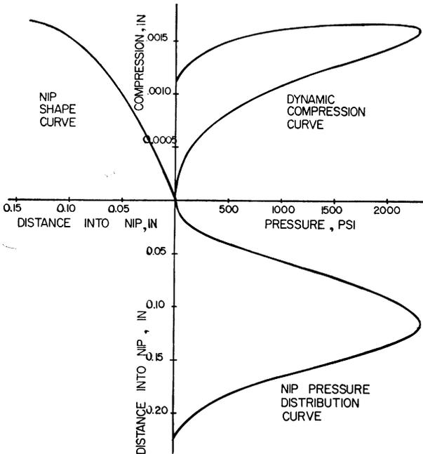
Fig. 41—Four quadrant graph giving nip pressure distribution—Grade D
