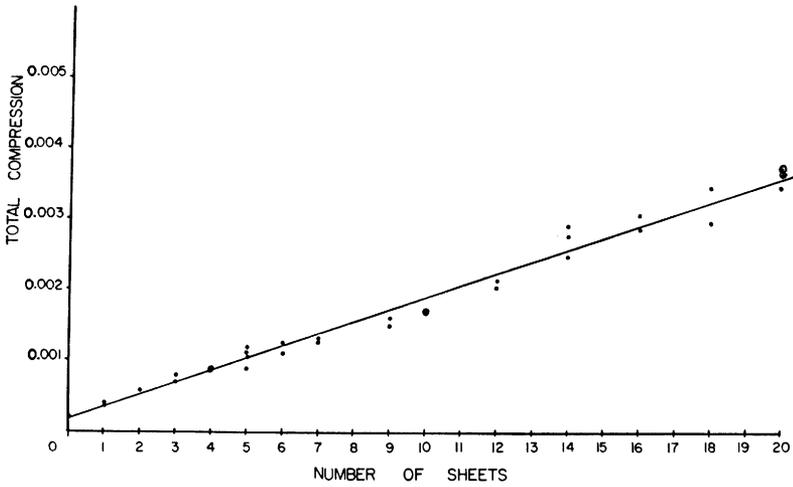
**Fig. 11**—Total compression as a function of the number of sheets tested
