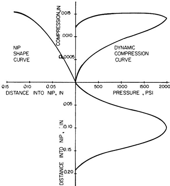
**Fig. 40**—Four quadrant graph giving nip pressure distribution—Grade C
