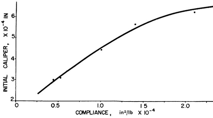
Fig. 15—Compliance as a function of caliper
