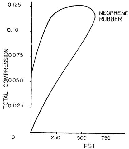
Fig. 6—Stress/strain curve for rubber block
