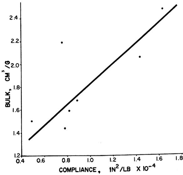
Fig. 16—Compliance as a function of bulk
