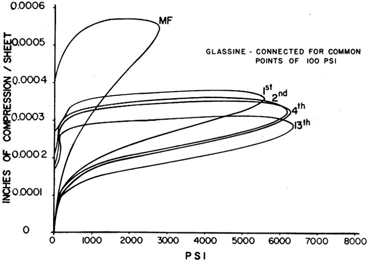
Fig. 25—The compression of glassine body paper sampled from successive nips of the supercalender
