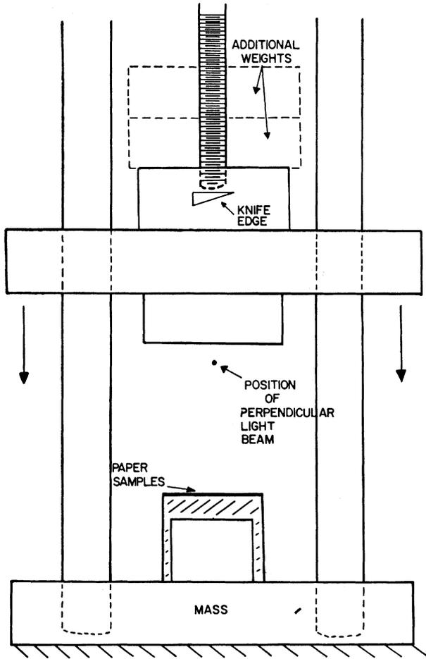
Fig. 4—Diagrammatic view of the free-fall hammer
