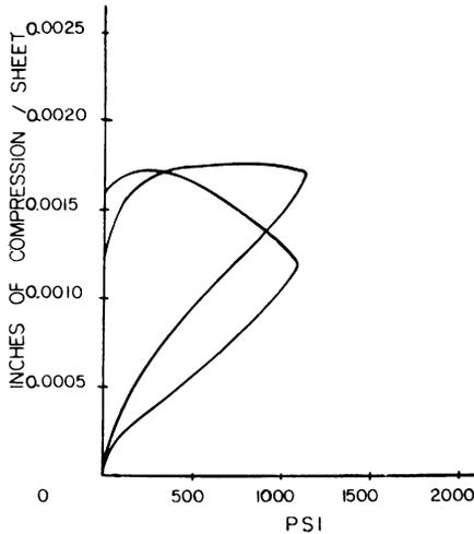
**Fig. 13**—Stress/strain curves in compression for 1 sheet and 20 sheets
