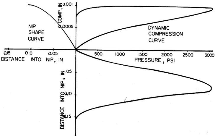
Fig. 39—Four quadrant graph giving nip pressure distribution—Grade B
