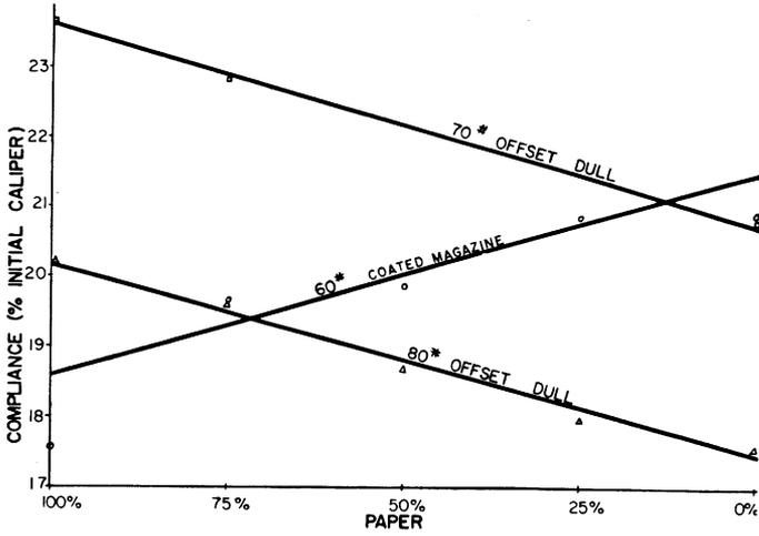
Fig. 30—Compression of paper and printing packing
