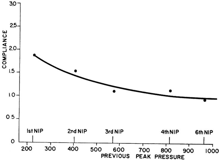
Fig. 17—Compliance as a function of previous peak pressure
