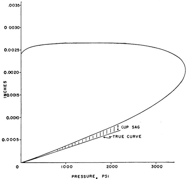
Fig. 8—Stress/strain curve for solid aluminium
