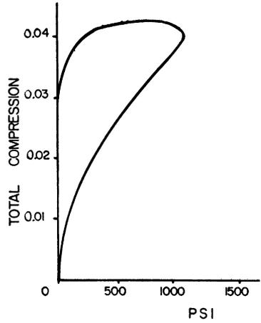
Fig. 34—Compression of newsprint packing plus a single sheet of high caliper newsprint
