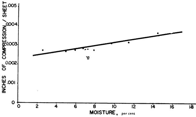
**Fig. 28a**—Static compression of groundwood as a function of moisture content
