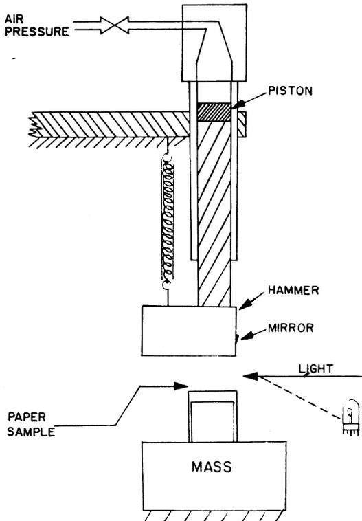
**Fig. 2**—Diagrammatic view of the air hammer tester
