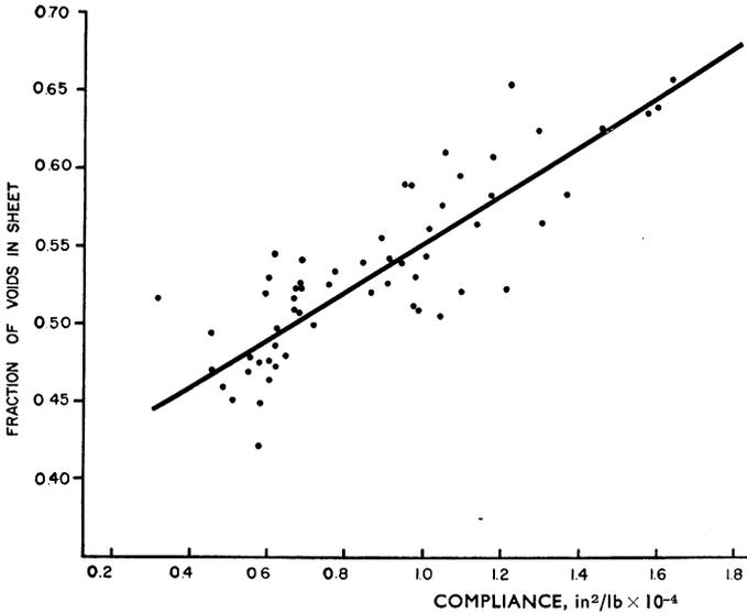
**Fig. 14**—Compliance as a function of sheet void space
