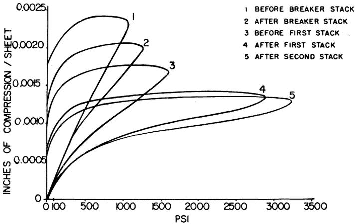
**Fig. 27**—Compression of paper at various stages made with a breaker stack
