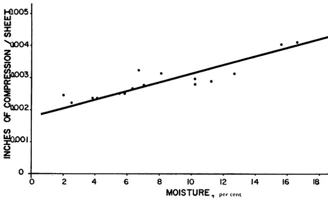
**Fig. 28b**—Dynamic compression of groundwood as a function of moisture content
