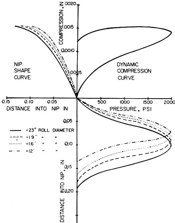
**Fig. 42**—Four quadrant graph giving nip pressure distribution changes for changes of roll diameter on the same paper
