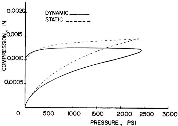
**Fig. 9**—Typical comparison of stress/strain plot in compression for static and dynamic tests
