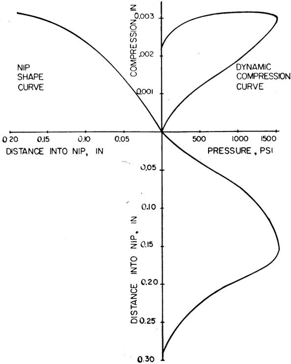
Fig. 38—Four quadrant graph giving nip pressure distribution—Grade A
