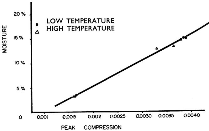
Fig. 29—Dynamic compression against moisture content at two temperatures
