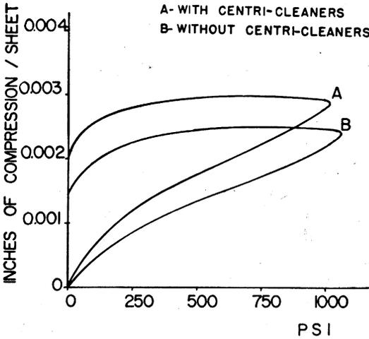
Fig. 26—Compression of newsprint made with and without centrifugal cleaners
