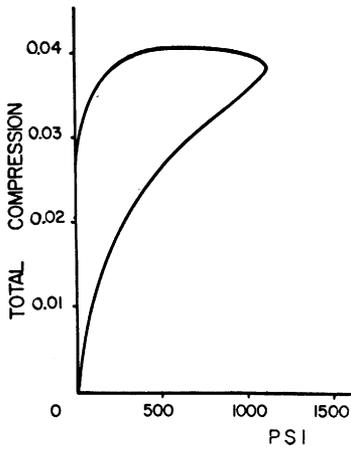
Fig. 33—Compression of newsprint packing plus a single sheet of low caliper newsprint
